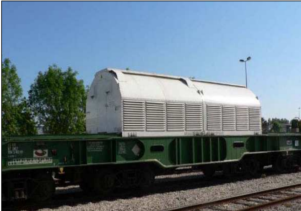
Figure 12. SNF Cask with Personnel Barrier Loaded on a Rail Car
