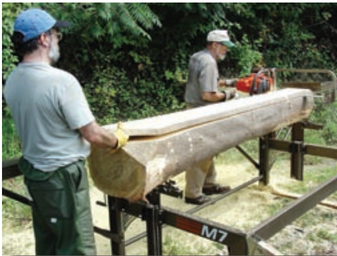
Figure 8: Cutting Ailanthus boards (Charlie Becker, left, and Tim Tigner, retired, of the Virginia Department of Forestry).
