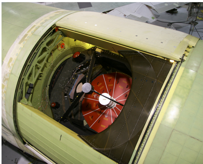
SOFIA's telescope in the 747's fuselage.
