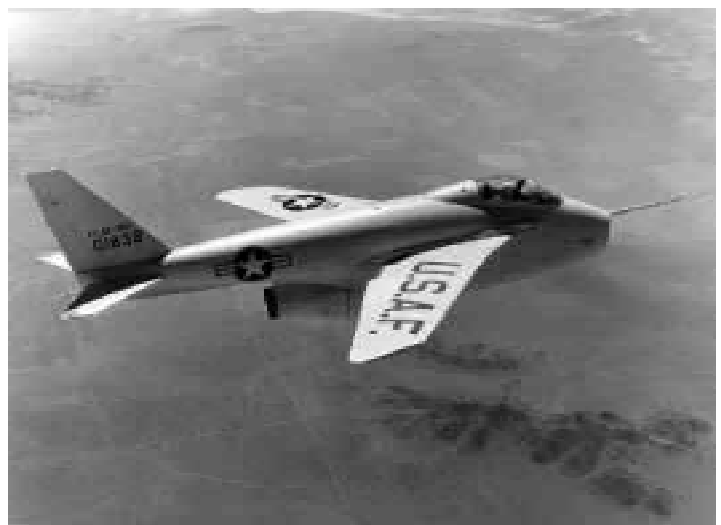
NASA Photo E-17351. The X-5, which proved the viability of variable-sweep wings.
