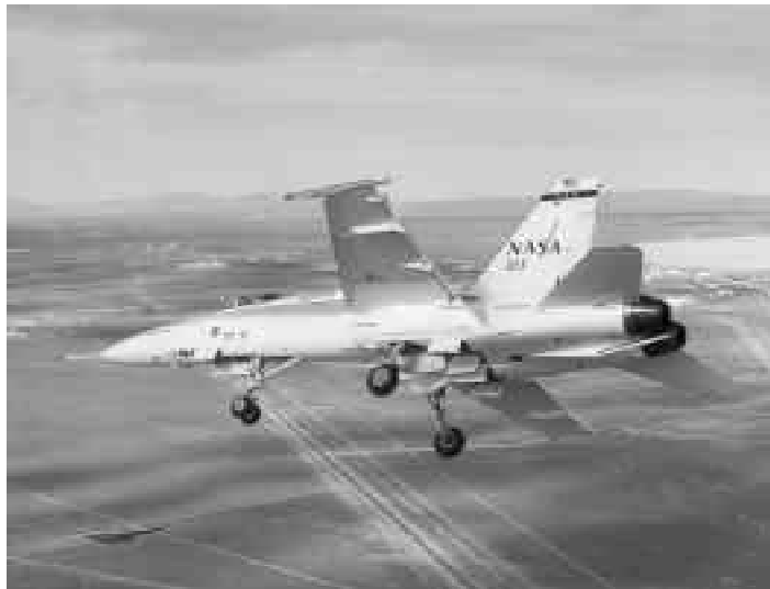
With landing gear and flaps down, NASA Dryden's Active Aeroelastic Wing F/A-18A research aircraft rolls towards final approach to the Edwards Air Force Base Runway at the end of a test flight. NASA Photof: EC03-0039-7.
