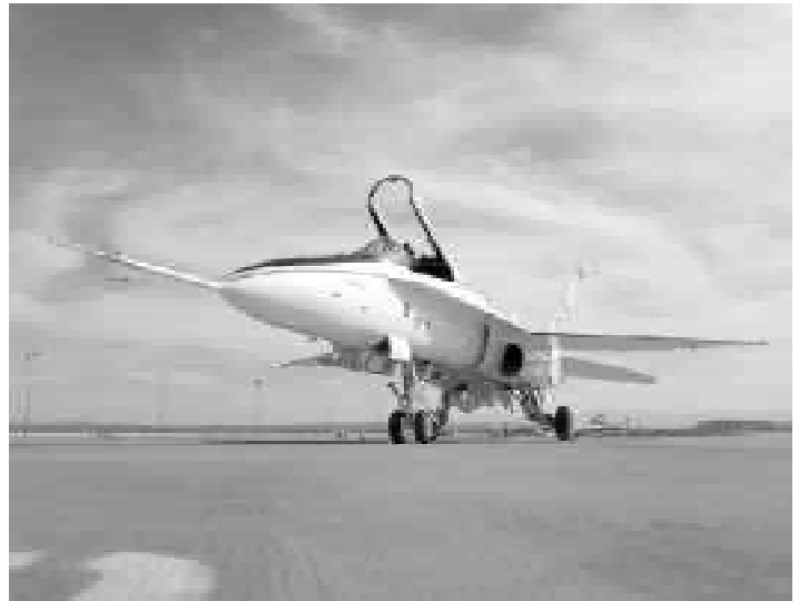
With a long flight data probe extending from its nose, this F/A-18A has been modified to conduct flight research in the Active Aeroelastic Wing (AAW) project at NASA's Dryden Flight Research Center, Edwards, California. NASA Photo: EC01-0288-5.
