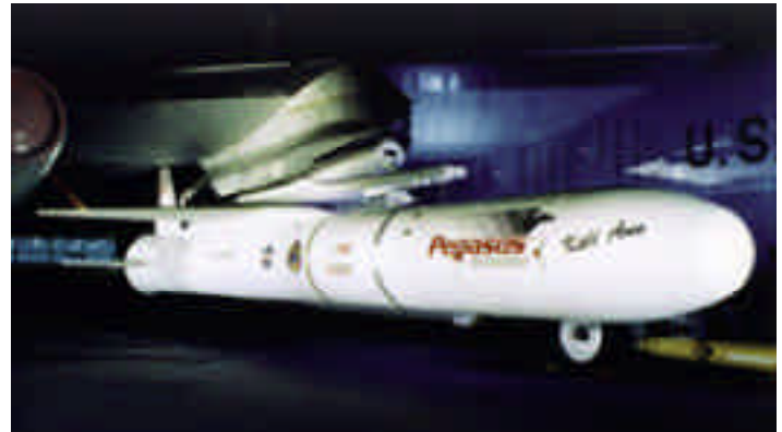
The Orbital Sciences Corp.'s Pegasus booster rocket is mated to Dryden's B-52. Orbital's L-1011 now serves as the Pegasus mothership.
