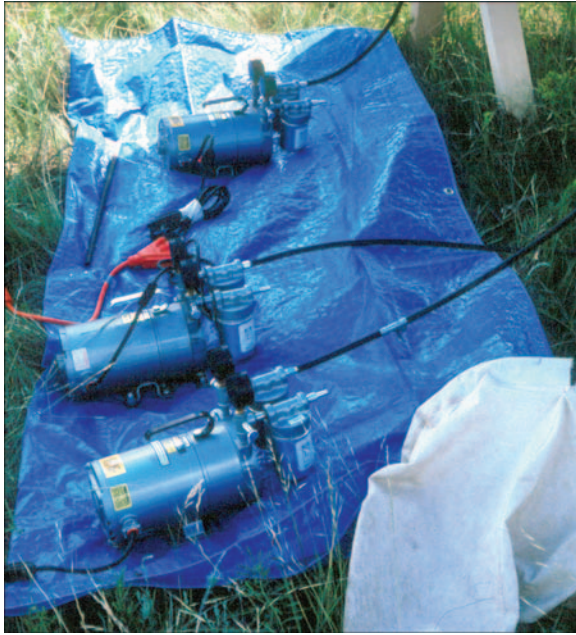
Figure 60. Electric vacuum pumps for sorting collected Aphthona adults. USDA-APHIS.
