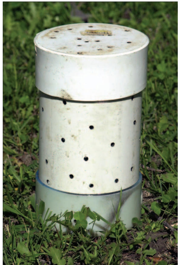
Figure 62. Passive Aphthona adult sorter, made from a length of 6-inch-diameter PVC pipe. Field-collected material is placed inside the pipe, and flea beetle adults crawl out the 3/16" holes. USDA-APHIS.
