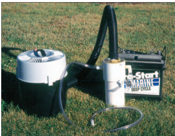
Figure 61. Small collecting vacuum that is powered by a 12-volt car battery and used to sort Aphthona adults under field conditions. USDA-APHIS.
