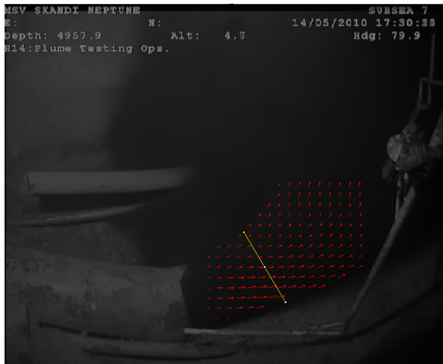
Figure 3: Displacement (or velocity) field and plume diameter measurement area. The average velocity is 7.52 in/sec and the plume diameter is 24.53 in along the yellow line.
