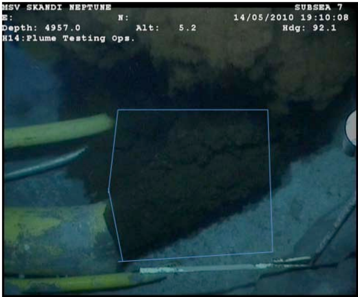
Figure 4: Definition of the Region of Interest in the images from the riser pipe's exit.
