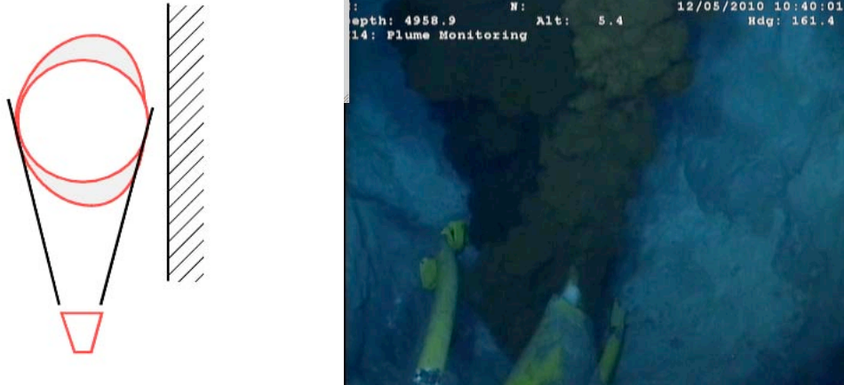
Figure 8: Top view schematic illustrating geometric correction due to wall effects.
