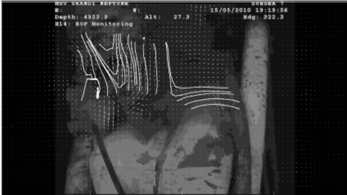
Figure 3: Sample PIV/LPT results for J_1 . The images in Fig. 2 are processed.
