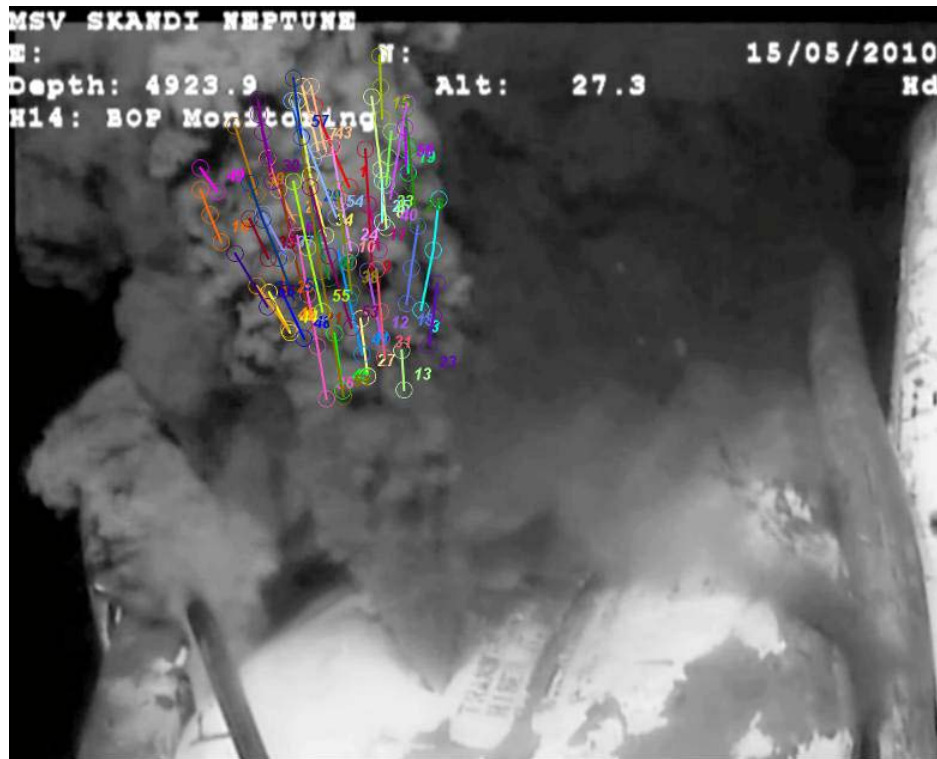
Figure 12: Feature tracks manually identified in the main jet of the Riser Kink Jet. (The trajectories of features shown in this image were pseudocolored randomly so they are easier to see. The colors do not represent velocity magnitude.)
