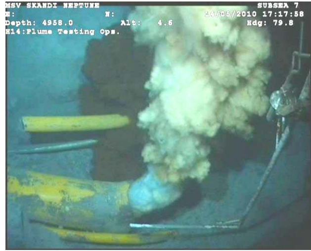
Figure 5: Riser End Jet when gas dominates the flow.
