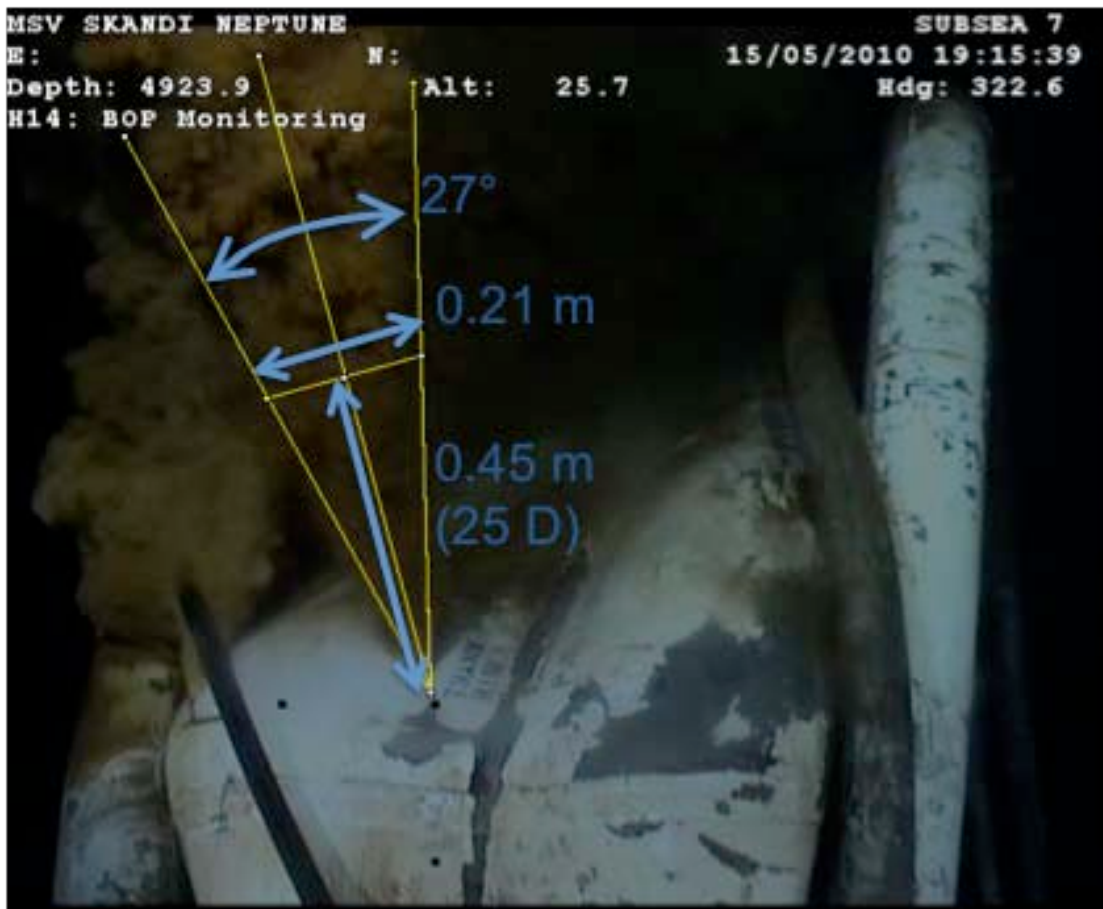
Figure 15: Sketch of the location of PIV measurements in the main leak on the kink at the top of the BOP. The jet is still momentum dominated (buoyancy effects not considered).
