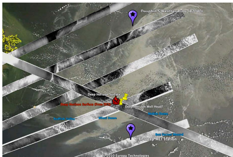
Figure 21: Overlay of AVIRIS Quicklook images of flight data for May 17 th , 2010, showing flightlines with MODIS data illustrating similarity and evolution of spatial features.
