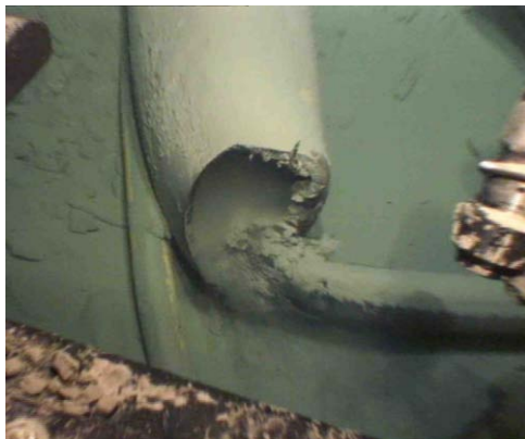
Figure 6: Photo supplied by BP on June 12 showing the exit of the end of the riser after oil had stopped flowing because the riser was cut above the BOP.
