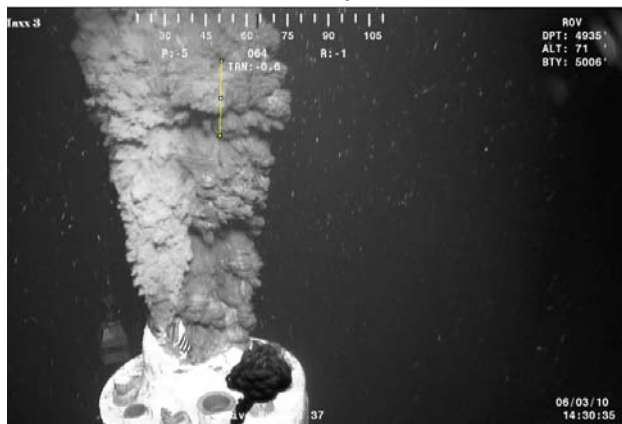
Figure 14: Hand analysis of features in the post riser cut plume. Yellow line shows feature tracked across a number of frames, which is noted above each figure as the delta time.
