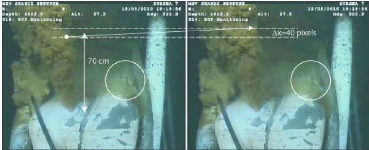
Figure 2: Two successive images from a video sequence (24 fps), showing the advection of large structures downstream of J_1 . Circles mark a group of dark patches that can be tracked individually. Individual frames are 880 pixels wide and 720 pixels high; the length scale: 1 pixel = 1.6 mm.
