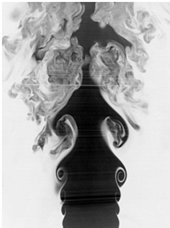
Figure 10a: Planar Laser Induced Fluorescence (PLIF) of a water jet injected into still water at Re=6000 . Image shown is a negative.
