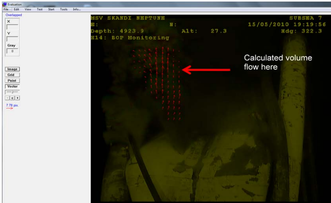
Figure 4: Velocity field for one of the jets at the location of the kinked riser and location where volume flow rate is calculated.
