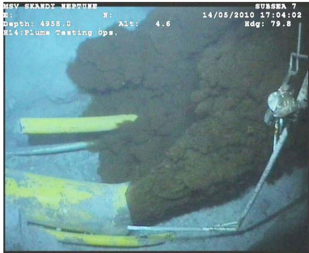
Figure 4: Riser End Jet when oil dominates the flow.
