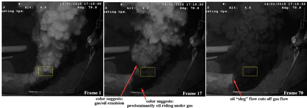
Figure 1: Plume of oil and gas escaping the riser pipe showing the three flow types, gassy, transition, and slightly oily. Also shown is the location of interrogation window.
