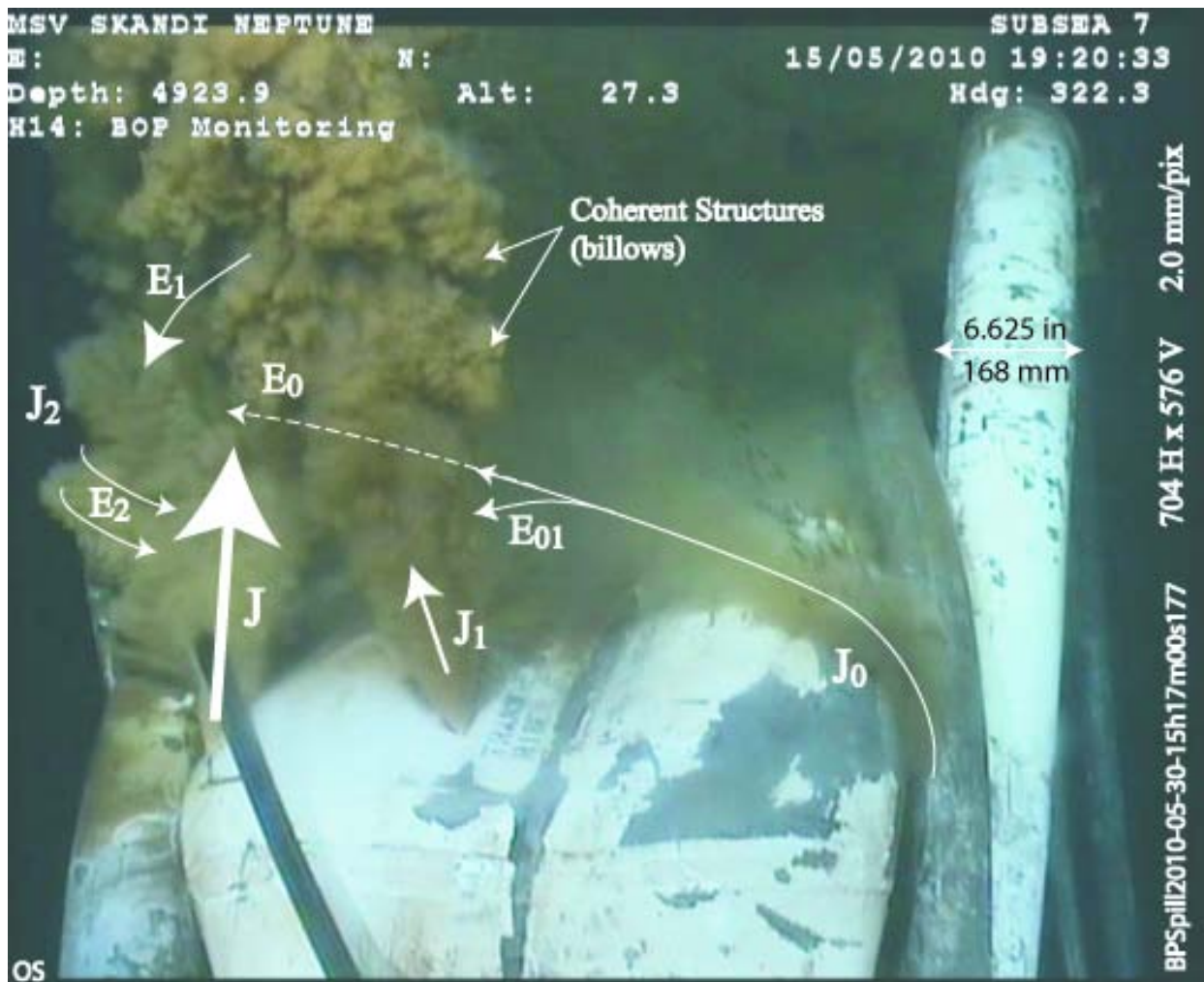
Figure 1: Summary of observations of the discharge flow field at the kink. J-jet, E-entrainment. The picture is 704 pixels wide and 576 pixels high; the length scale: 1 pixel = 2.0 mm.
