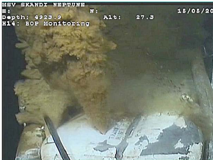
Figure 2: Several jets emitting from openings in the Riser Kink area above the BOP.
