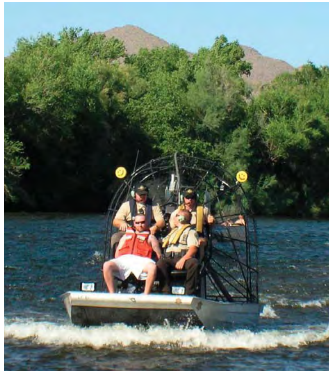
The Maricopa County Sheriff's Office operates one of the few airboats in the state of Arizona. The shallow draft of airboats makes them an ideal platform for accessing the shallow and hard-to-reach areas of the Lower Salt River.
