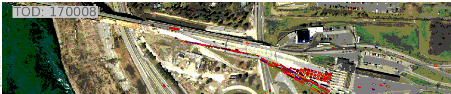
Simulated traffic queue at U.S. Customs in Lewiston, NY, near Niagara Falls. Red blocks represent vehicle in line.
