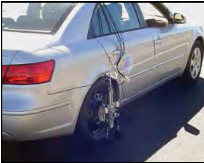
Vehicle equipped to gather Traffic Noise Model data. (Volpe Center photo)
