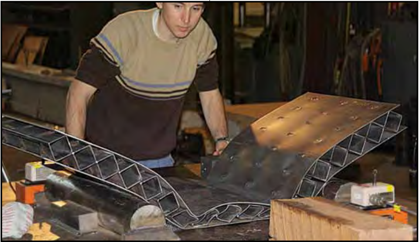
Volpe Center mechanical engineer Michael Carolan inspects a prototype panel after a structural bend test at the Lehigh Center for Advanced Technology for Large Structural Systems. (Volpe Center photo)
