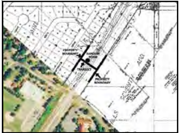
Example of a ROW property map overlaid on an aerial photograph to determine and measure distances between boundaries. (Volpe Center image)
