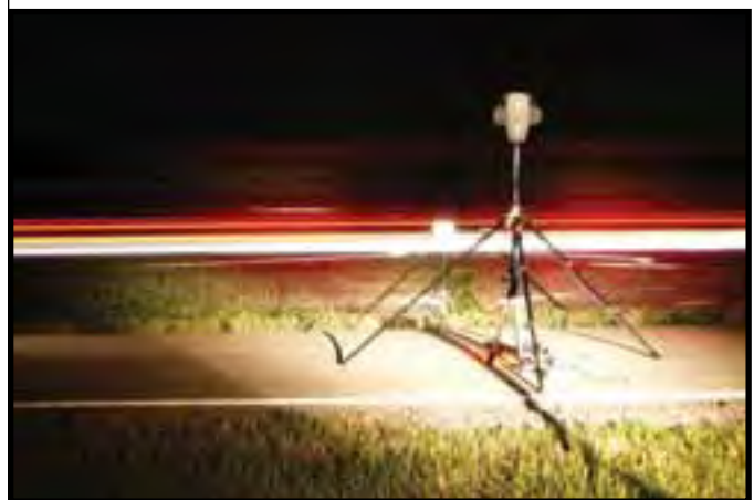
The Volpe Center recorded the sounds of hybrid-electric and internal combustion engine vehicles in various speed and operating modes and used the recordings to examine the auditory detectability of vehicles by vision-impaired pedestrians. (Volpe Center photo)
