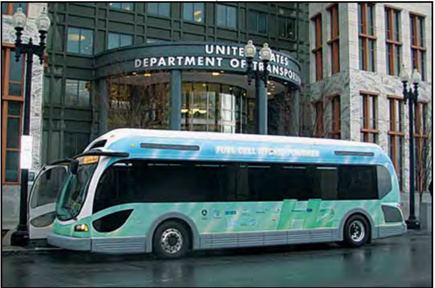
NFCBP battery-dominant hybrid hydrogen fuel cell transit bus outside U.S. DOT headquarters in Washington, DC. (Photo courtesy of the National Fuel Cell Bus Program)
