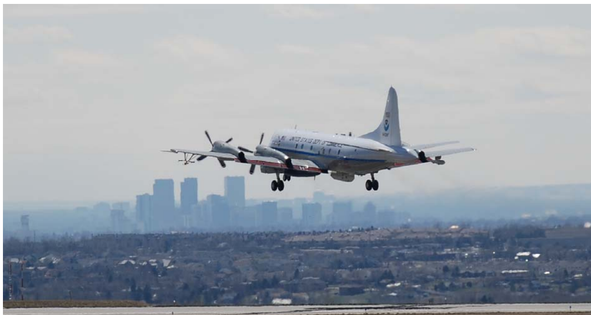
Fig 1. A NOAA WP-3D Orion research aircraft, equipped as a flying air chemistry laboratory departs on a research mission.
