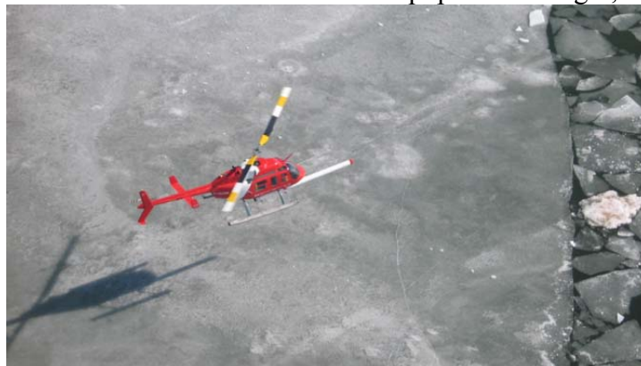
Figure 2.3.2. IcePIC hard-mounted on the front of a helicopter flying over sea ice
