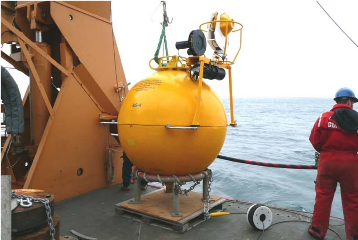
Figure 2.5.1. The Arctic Winch attached to the top float of a subsurface mooring being deployed in the Beaufort Sea. The sensor suite is attached to the small yellow buoyant float which sits in a cradle above the data logger (black cylinder), next to the winch spool and motor (black disk).
