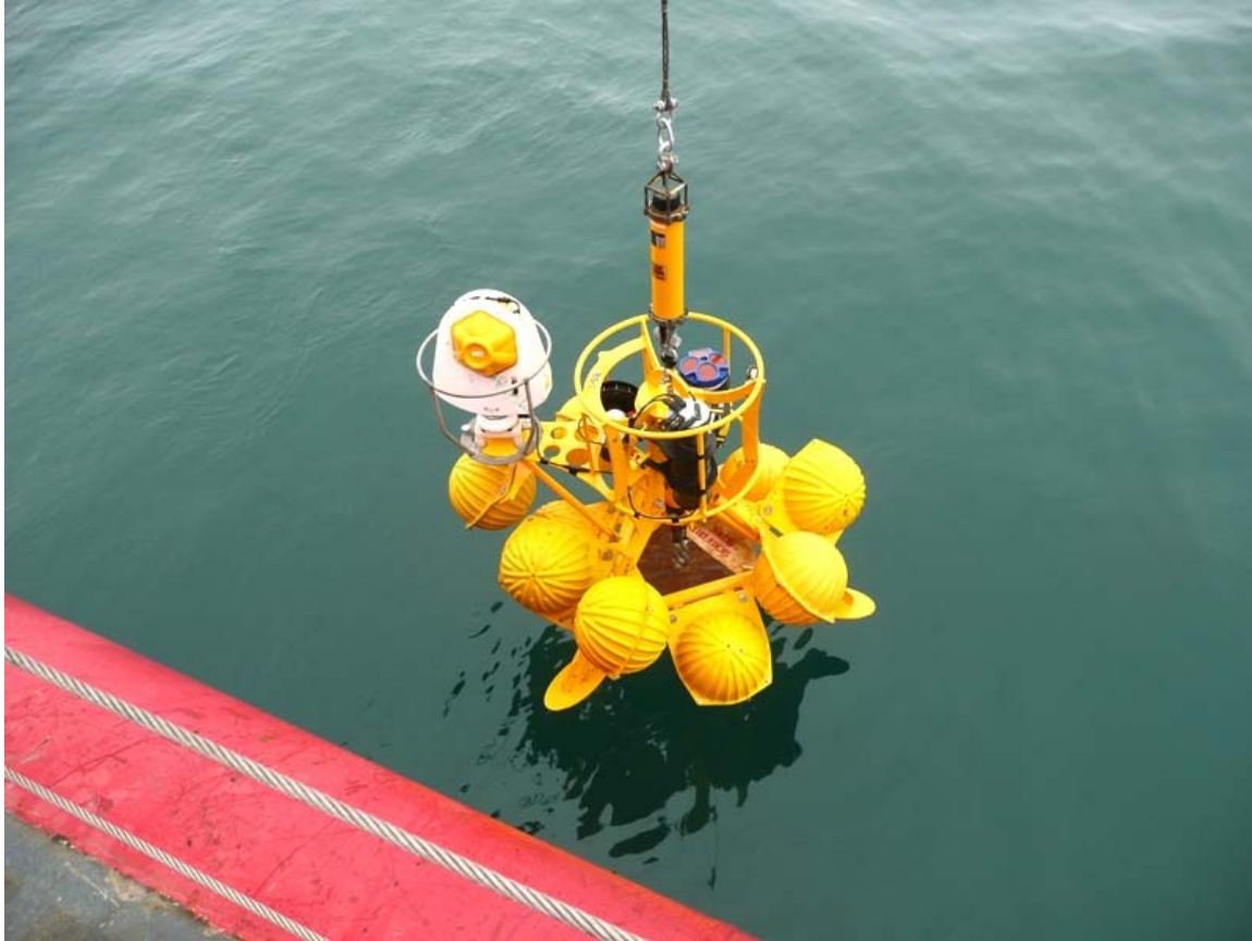
Figure 2.5.2. The Arctic Winch attached to a tripod being lowered to the seafloor on the continental shelf in the Beaufort Sea.
