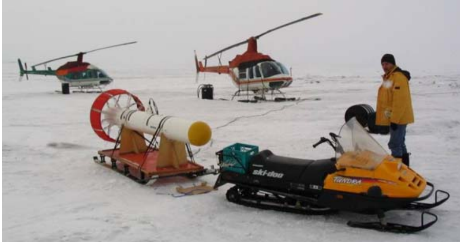
Figure 2.3.3. EM Bird on sled behind snowmachine with cable to helicopter.
