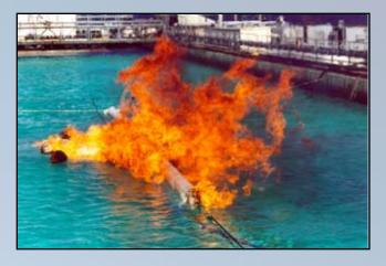
and, (viii) destructive testing was used to estimate the operational life of the flexible connector sections and the tensile strength of several key load-bearing components. Finally, the design of the boom was refined and final detailed engineering drawings and a technical paper was produced. The boom successfully passed all the required engineering and burn tests. The final design is freely available to interested parties. TAR Project 289. http://www.mms.gov/tarprojects/289.htm.
