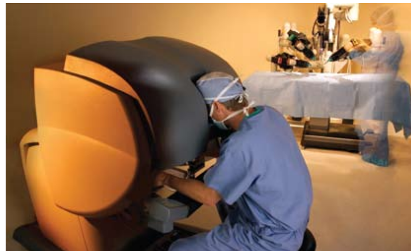
Surgeons can manipulate the da Vinci surgery robot from a remote console in the OR while seeing the surgical field in a magnified, dimensional view.
