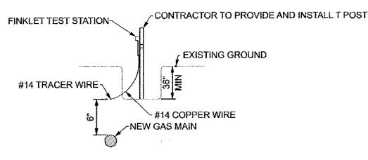
1, #1 ZINC ANODES ARE TO BE PLACED AT 500' INTERVALS WITH A 14 GAUGE (#14) COPPER WIRE CONNECTING THE ANODE TO THE TRACER WIRE. EVERY OTHER ANODE MUST BE CONNECTED TO A TEST STATION.
