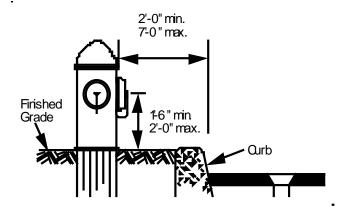
507.5.1.3 Fire Hydrant Location and Spacing. Fire hydrants shall be located and spaced per the following criteria:
