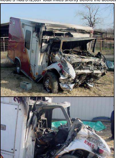
The engine and transmission were replaced in July and August 2002, respectively. The vehicle underwent modifications based on Ford factory recall # 98S08 on August 12, 2002. The recall was because of fuel line chafing in similar vehicles which could cause a fuel leak or fire.
