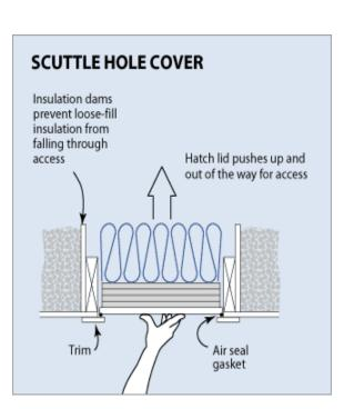
For air sealing, weatherstripping can be installed either on the hatch itself or on the inside of the trim or base where the hatch rests. Adding a latch bolt will help ensure a tighter seal.
