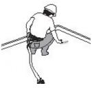
The fall restraint system's anchor must support at least 3,000 lbs. Otherwise, it must be designed, installed, and used under the supervision of a qualified person.
