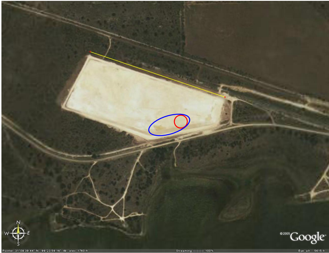
Note: Yellow line along the pond is ~582 m (1,911 ft) long; blue outline shows water body at time of sampling Figure 12-14. Aerial view of the evaporation pond of City of Brady desalination facility showing sampling location (courtesy of Google Earth)
