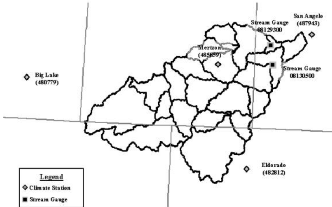
Figure TBN-7. Climate and Stream Gauge stations in Spring and Dove Creeks.
