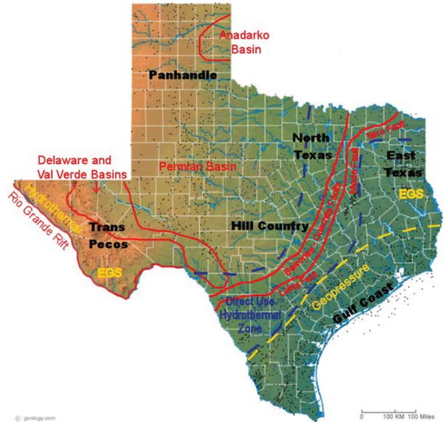
EXHIBIT 7-3 Generalized geographic and geothermal location map. Wells locations shown by blue dots (less than 4000 feet) and black dots (greater than 4000 feet). High temperature resources are shown in yellow text and low to intermediate temperatures are in blue. Geologic features are highlighted in red. Map produced by the SMU Geothermal Laboratory.
