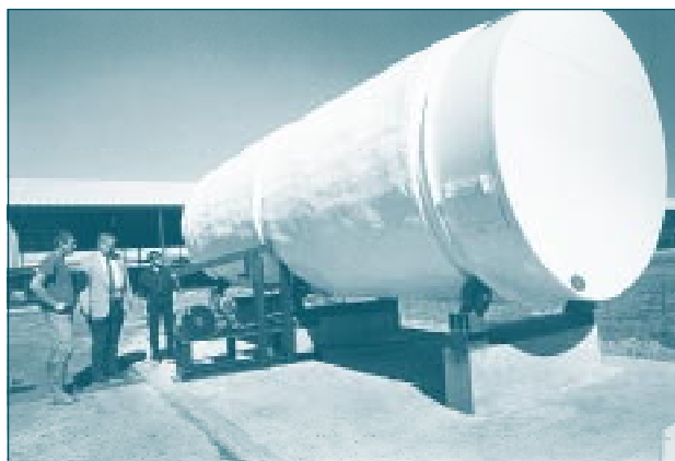
Compost was produced in this commercial composter from animal wastes generated at a 400-cow dairy. Building on the success of this project, the TNRCC and the TSSWCB are working to develop markets for composted animal waste that will move nutrient-rich material out of watersheds impacted by intensive agricultural land use.
