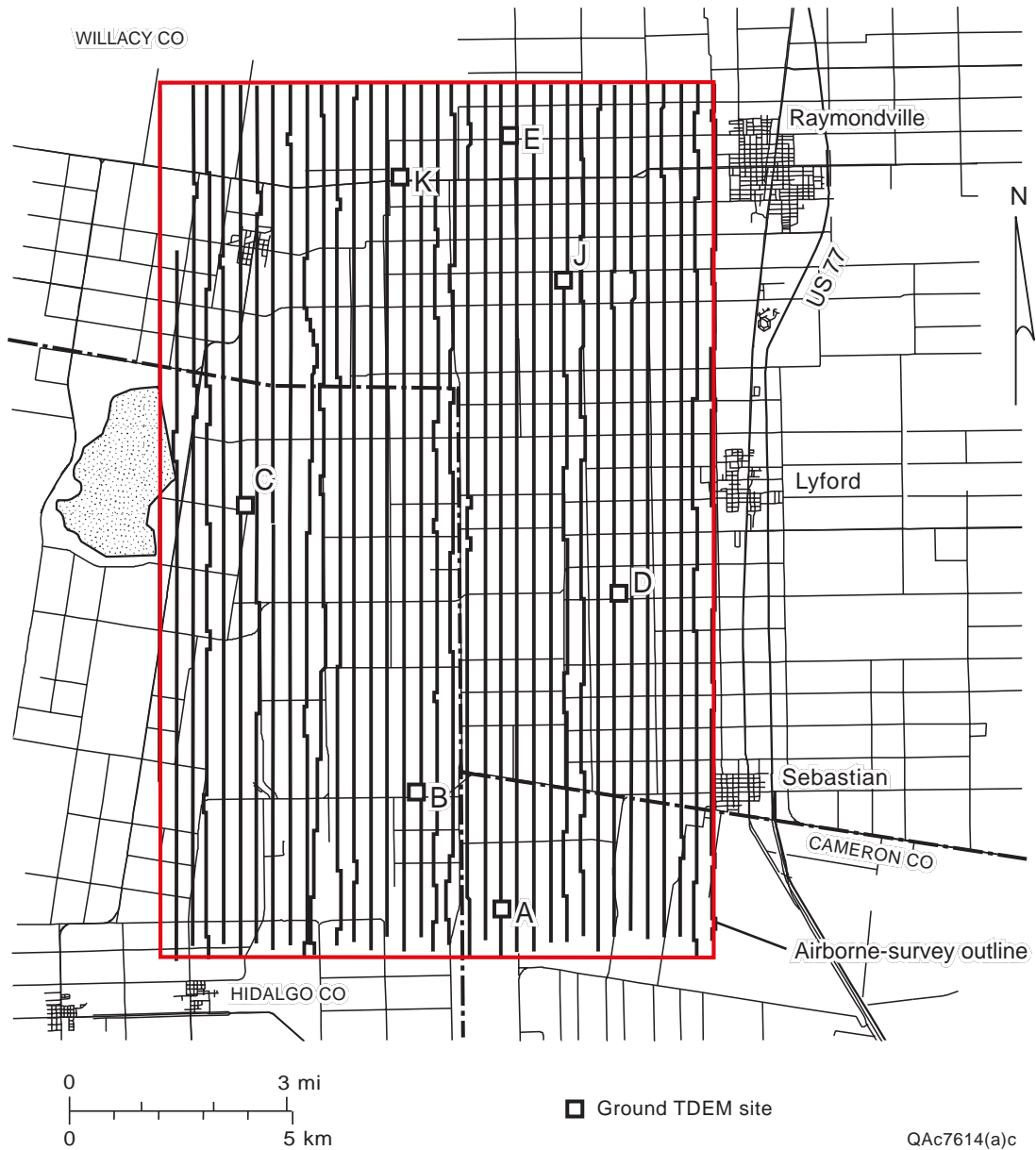
Figure 10. Flight lines flown by World Geoscience over the Stockholm area in August 1999. Also shown are ground TDEM sites.
