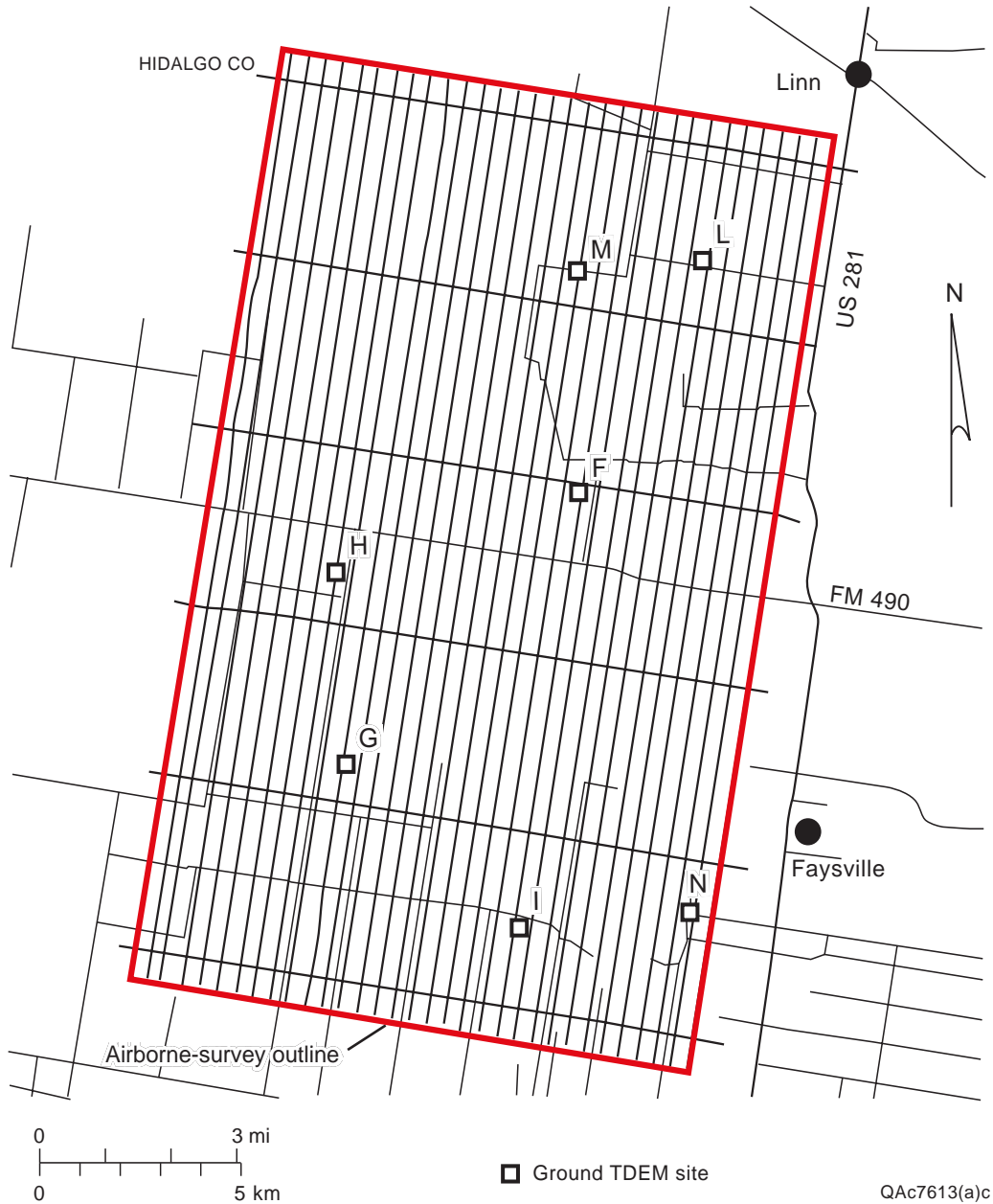
Figure 12. Flight lines flown by Geoterrex over the Faysville area in October 1999. Also shown are ground TDEM sites.
