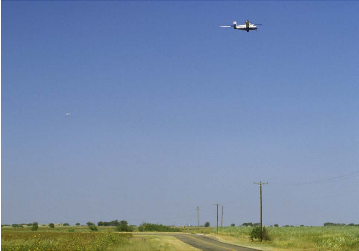
Figure 11. World Geoscience's QUESTEM airborne TDEM system operating above the Stockholm area, August 5, 1999. The receiver trails the aircraft. Photograph by David M. Stephens.
