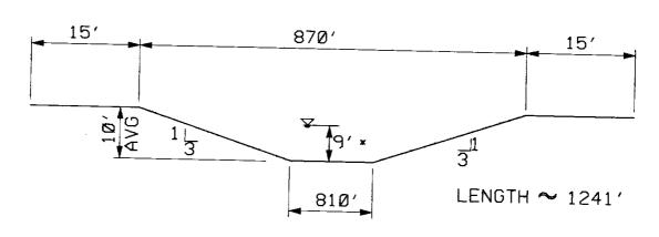
\* HIGHWATER ELEVATIONS ARE BASED ON HCFCD FREEBOARD REQUIREMENTS
