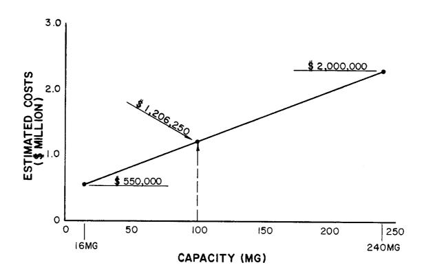
Estimated construction cost for a 100 mg interim balancing reservoir with 10' depth = \$1,206,250.
