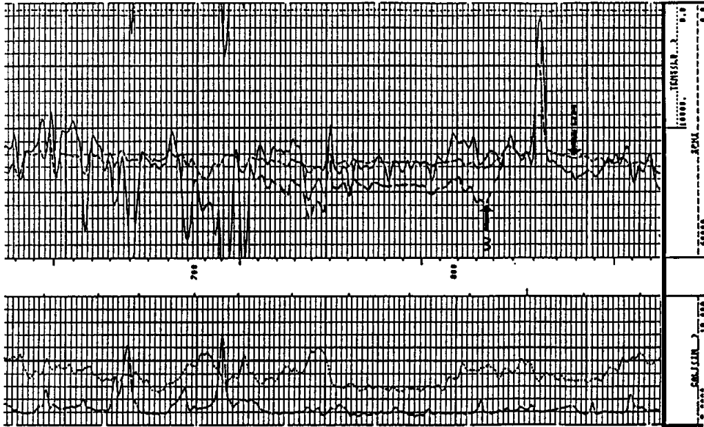
Figure 13-27 a & b. Comparison of the effect of compaction on porosities calculated with the Wyllie (W) and Raymer-Hunt (RH) transforms. At shallow depths (e.g. 750 to 790 feet) the Raymer-Hunt transform adequately corrects for a lack of compaction in the sandstones, while the Wyllie equation yields porosities that are too high. However, at deeper depths (e.g. 2600 to 2650 feet) the sandstones are compacted and both transforms calculate correct porosities. Density porosity is assumed to be true porosity. Figure 13-22 contains additional information on this well.
