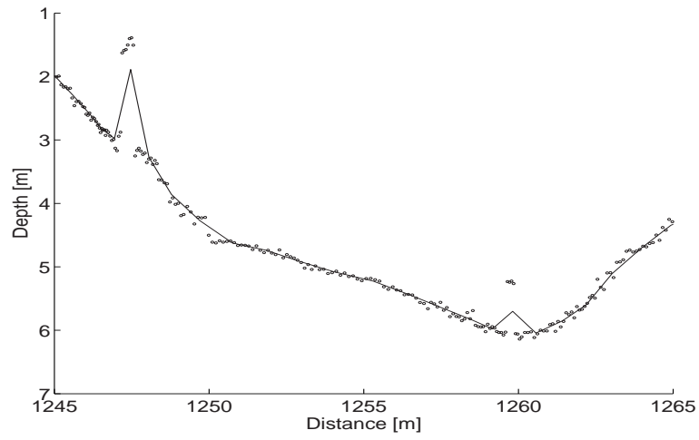
Figure 2.3: Distributed depth measurements along boat track are represented by points while the solid line is the averaged bathymetry.
