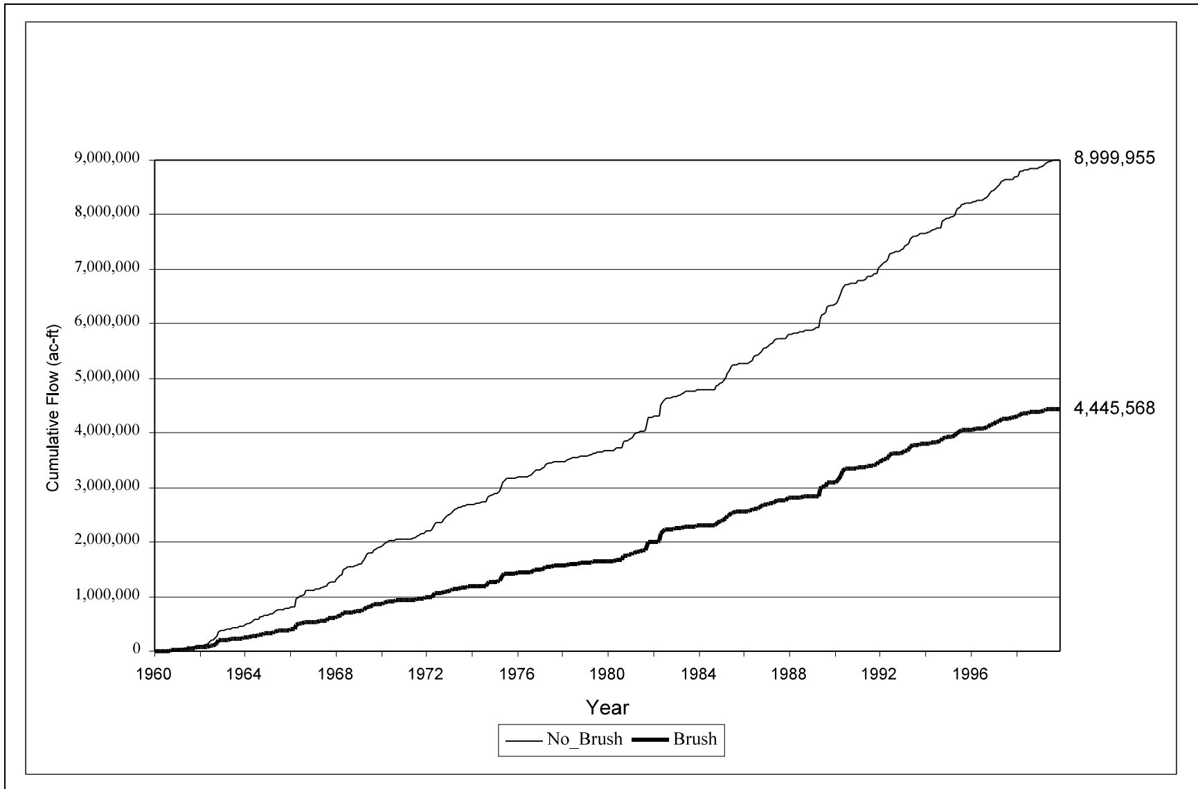
Figure 3-9. Predicted cumulative monthly stream flow into Lake Arrowhead for brush and no brush conditions.
