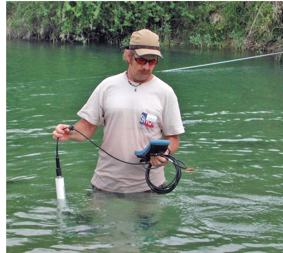
TCEQ SWQM staff member Bill Harrison uses the Hydrolab water quality monitoring device.
