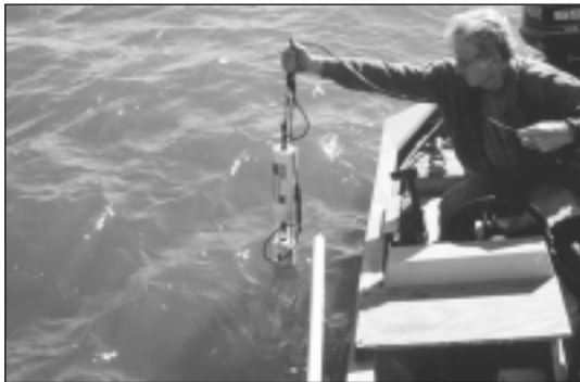
Surface water quality monitoring staff routinely collect field measurements, such as water temperature, pH, dissolved oxygen, and specific conductance.
