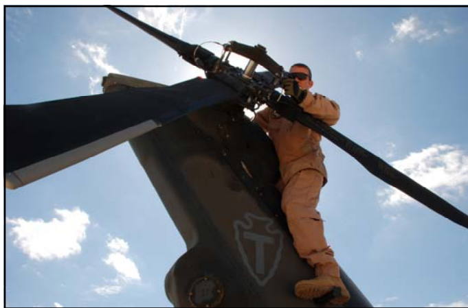
Lt. Col. Andrew Rochstein checking the tail rotor blades for excessive play and securing cable attachments on his UH-60 at the Austin Flight Facility.
