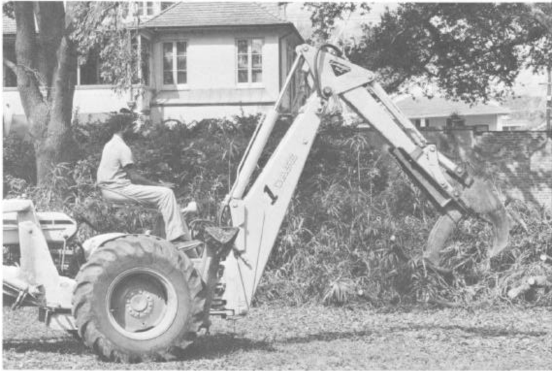
Figure 45. The "Claw" developed by the Corps for the truckloading of large tree limbs
