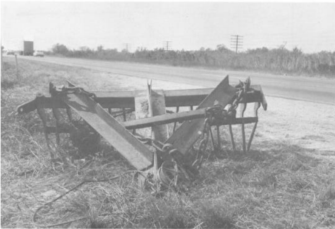
Figure 48. "Rake" developed by Corps personnel for collecting waterborne debris
