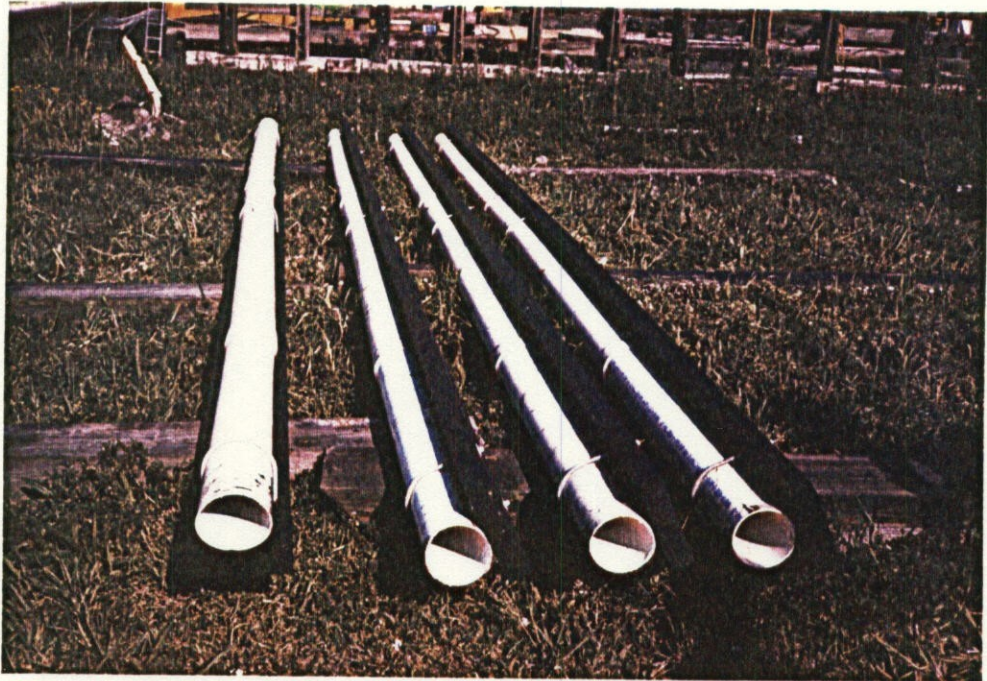
Photo No. 10 - Members of new cathodic protection system.
