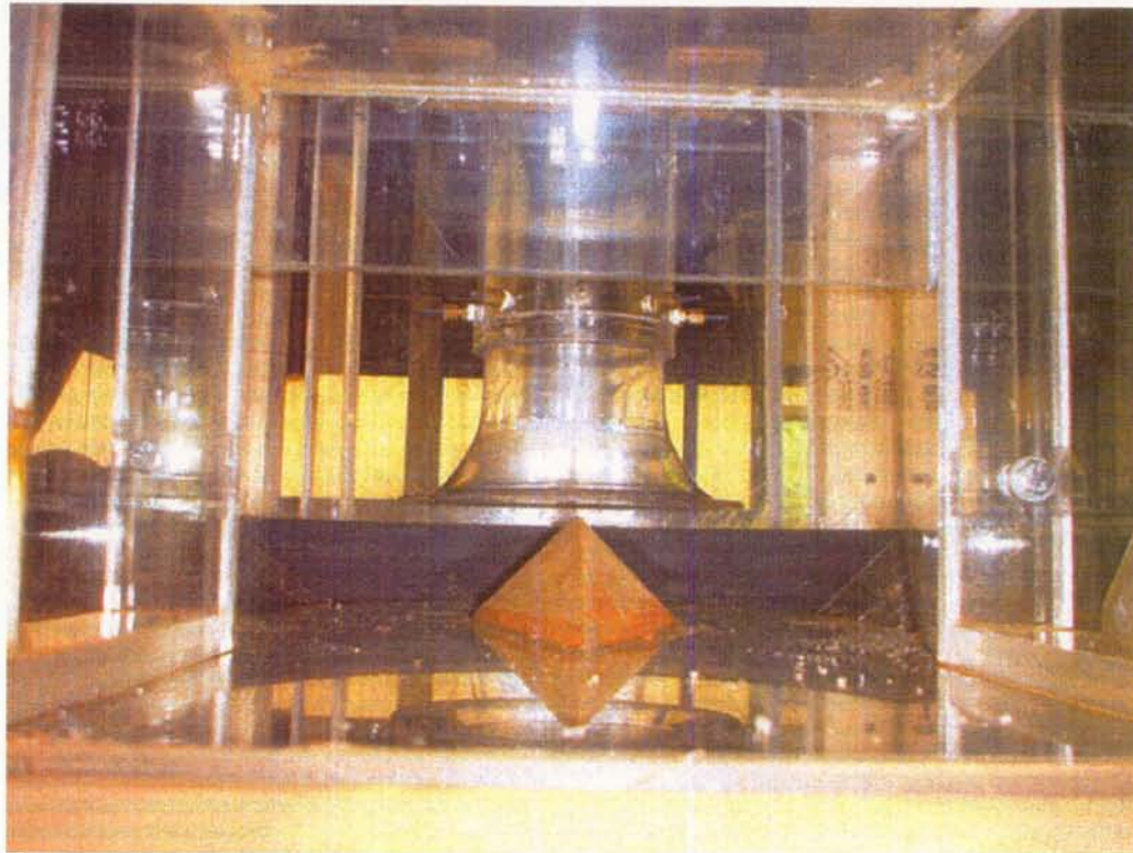
FIGURE A5 RECOMMENDED INTAKE BAY CONFIGURATION
