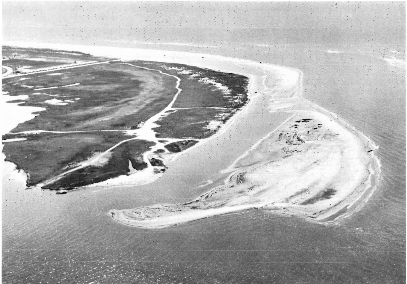
33 Photograph 17 Offshore bar in process of becoming attached to West end of Grand Isle
