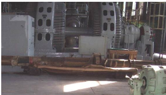
Photo 3 – Frequency changer motors.
