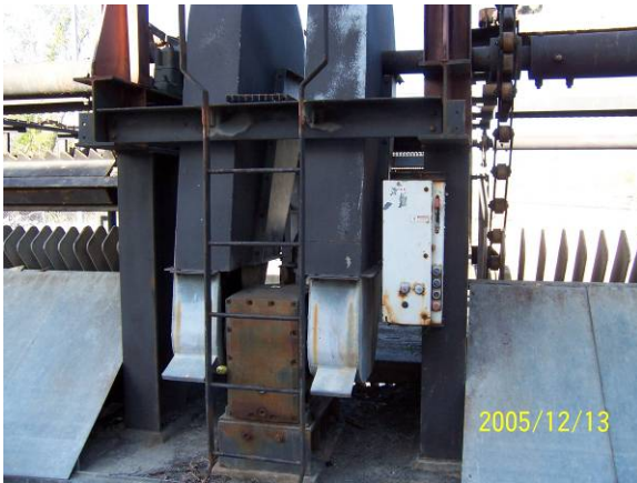
Photo 1—Damaged Control Panel for Trash Rack Photo 2—Damaged Diesel Engine
