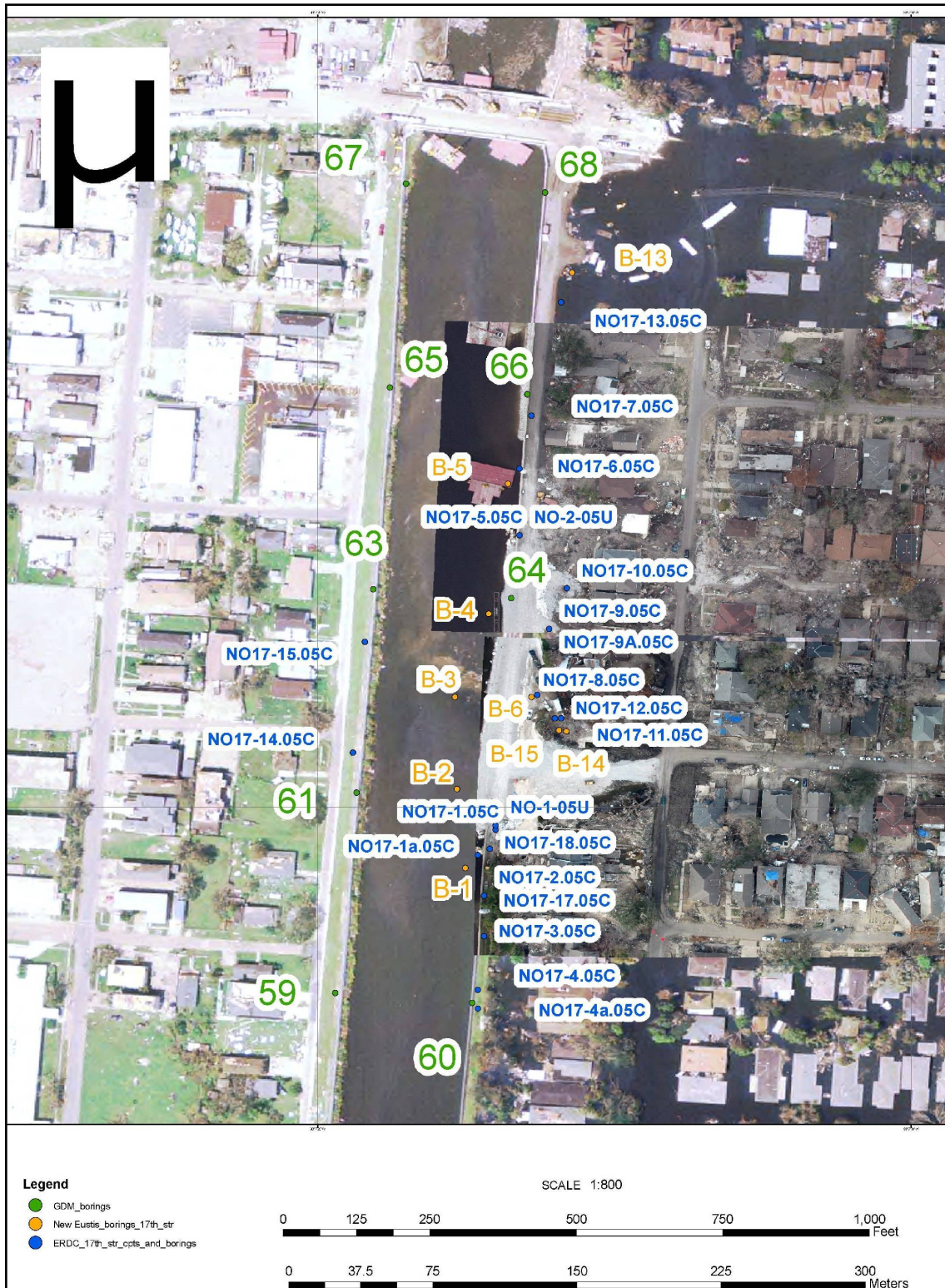
Figure VI-15. Boring and CPT Location Map
