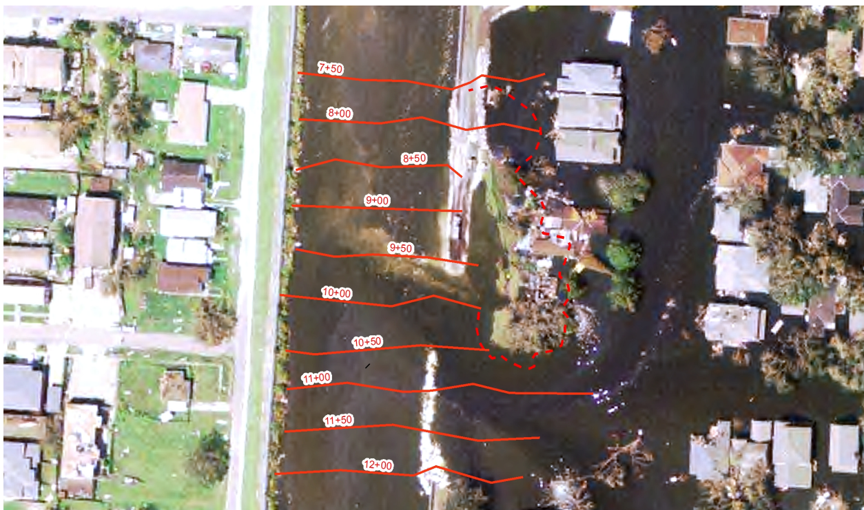
Figure VI-4. Location of multi-beam sonar survey cross-sections
