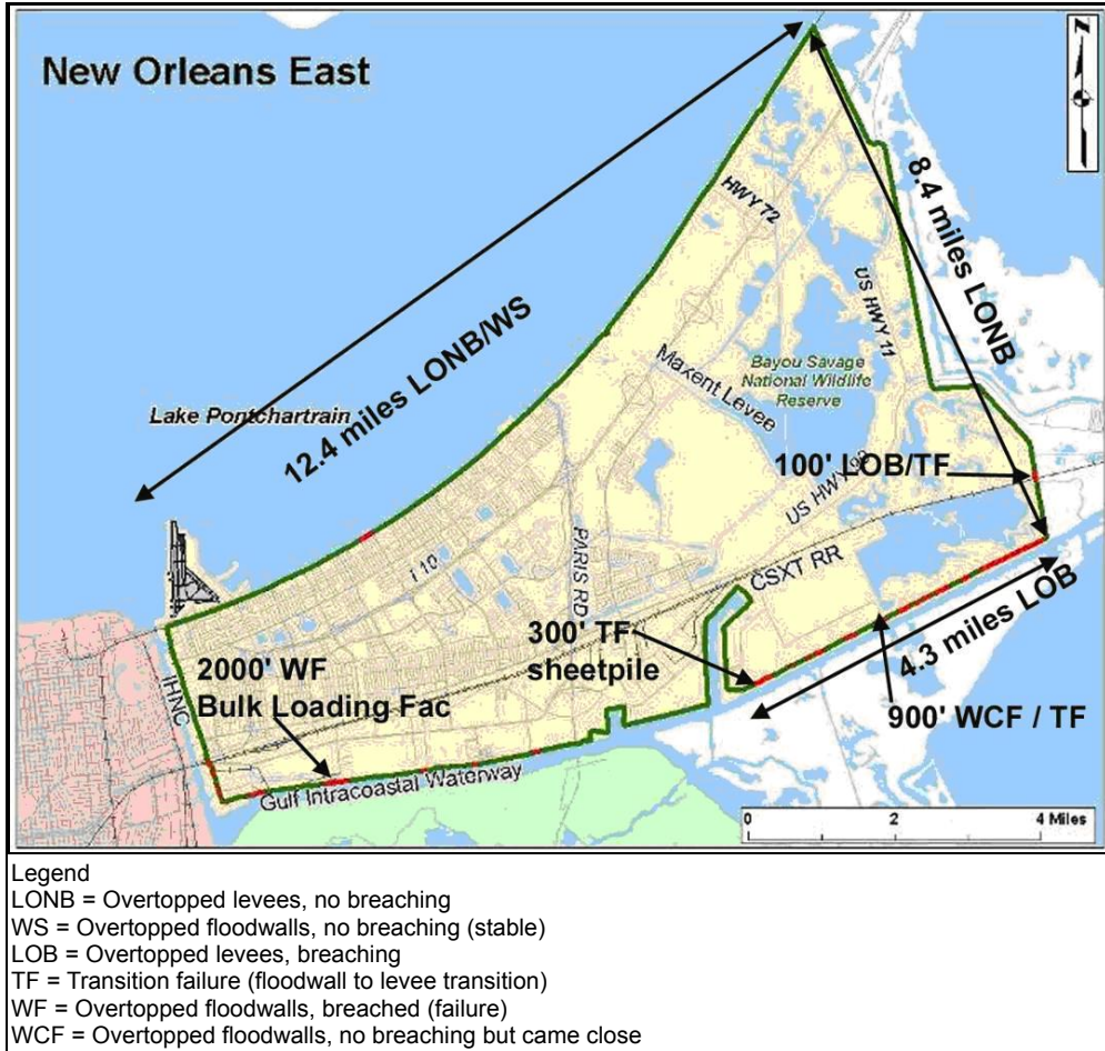
Figure VI-23. Generalization of levee and floodwall failures in the NOE basin
