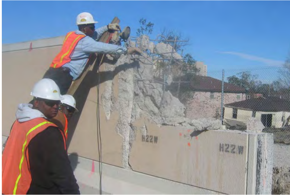
Figure K4-14. A portable electric bandsaw is used to cut rebar samples
