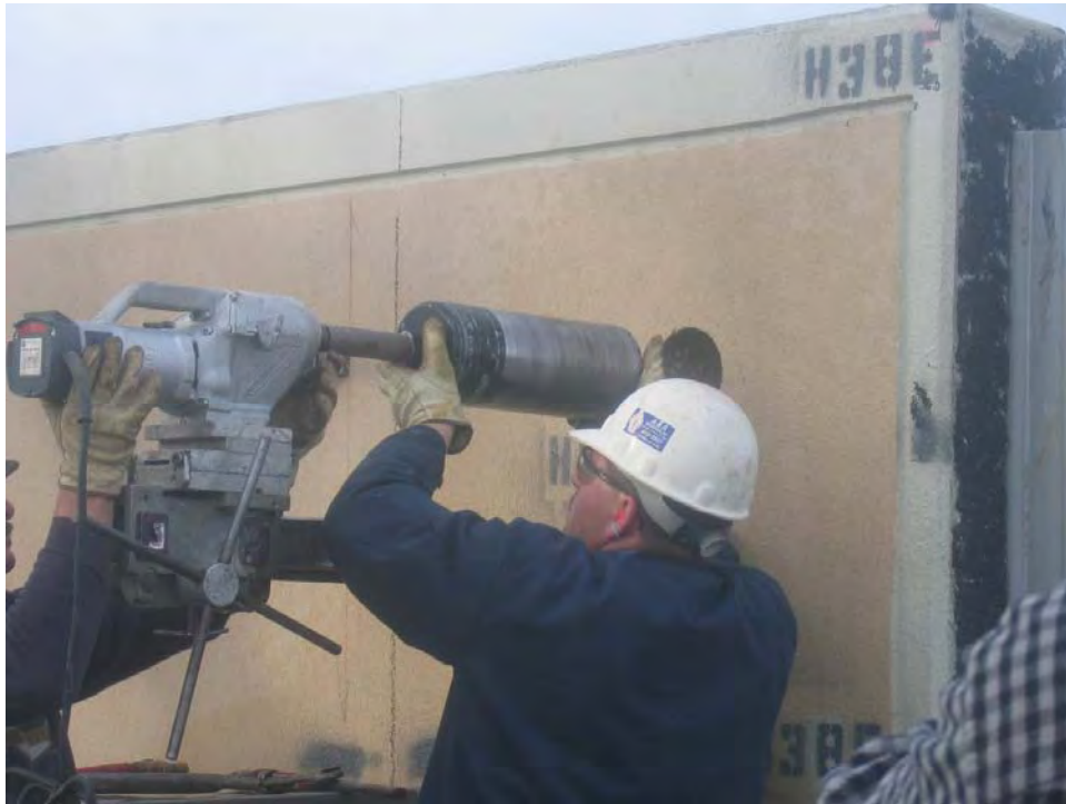
Figure K4-4. core being removed from panel H38
