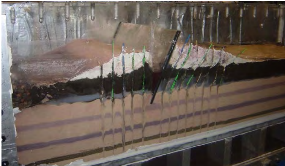
Figure K3-5. Rotation of the sheet pile wall in the London Avenue Trial Model
