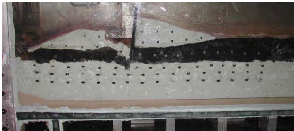
Figure K3-7. Sliding movement of the levee landward (to the right) observed at the completion of the 17th Street trial model test
