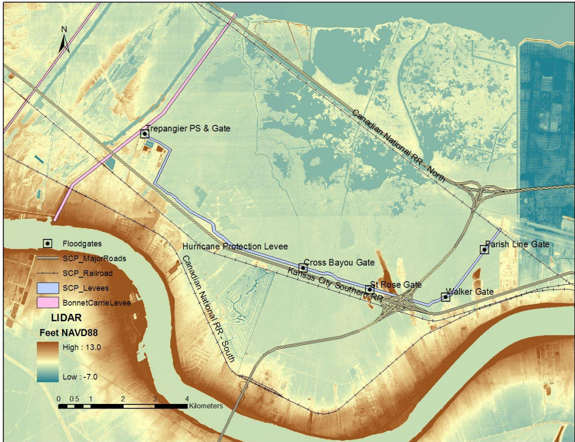
Figure 9-11. Levees, Pump Stations and Flood Gates
