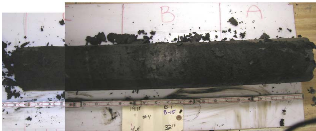
Figure 8c. Photographs of soil samples from B-15, samples 2 through 4, 0.5 to 8 ft depth; samples 2 and 3 from the levee fill, sample 4 from the swamp/marsh environment--note the high water content identified in Figures 8a and 8b, and the high organic content as indicated by the CHOA to CHOC designation for sample 3 (see Figure 1). Presence of wood pieces and roots are common in samples.
