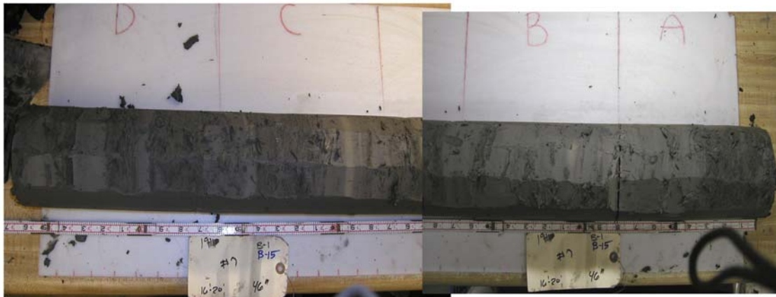
Figure 8d. Boring B-15, samples 5 (top), 6 (center), and 7 (lower); depths from 8 to 12 ft, 12 to 16 ft, 16 to 20 ft, respectively. See boring and lab logs in Figures 8a and 8b for descriptions. Sample 5 at top (right) contains the slip surface which is grey clay with distorted inclusions of peat in parts A and upper half of B. Shear zone is underlain by nearly 1 ft of peat (marsh deposits). Marsh deposits above and below grey clay layer have age date of 2,900 years. Lacustrine deposits begin in 5C at 10.6 ft. Note the sharp contact with the lacustrine deposits, and the distinct change to soft grey clay with trace organics and most importantly shell fragments (white specs) and silt and fine sand laminations. Note the change in water content between marsh and lacustrine in boring and lab logs. Bioturbation occurs in upper part of the lacustrine stratigraphic unit.
