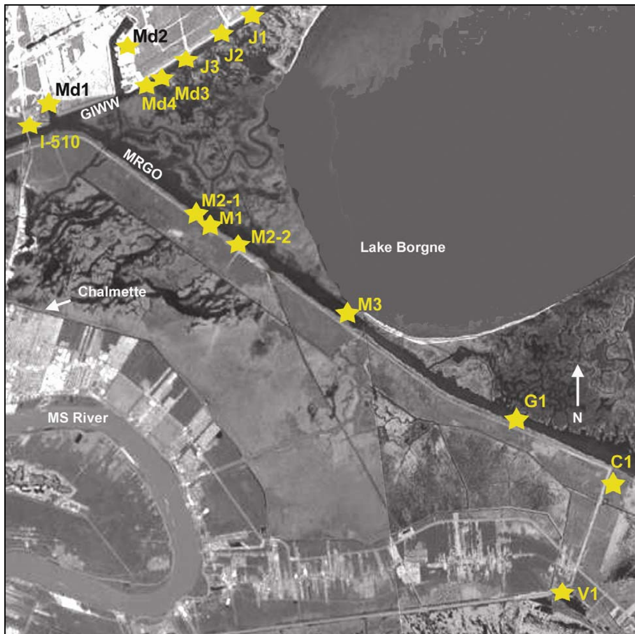
Figure 47. Overview of Jet Index testing sites (15 total) located on New Orleans East and St. Bernard levees.
