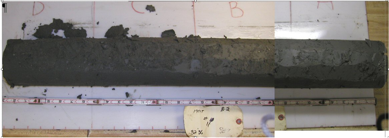
Figure 7f. Boring B-14, sample 11; depth from 32 to 36 ft, view of lacustrine grey clay, note the shell fragments near base of sample (left side), overlying and merging with the relic beach sand at 35 to 40 ft (Figure 3). See Figure 7b for lab summary descriptions.
