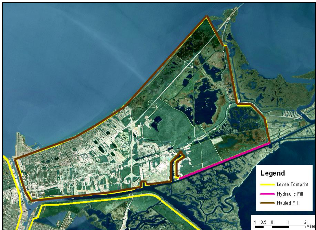
Figure 13. NOE Levee construction materials (from USACE DM NOE Back Levee, Citrus Back Levee, South Point to GIWW levee, Lakefront Levees, IHNC levees after 1969)
