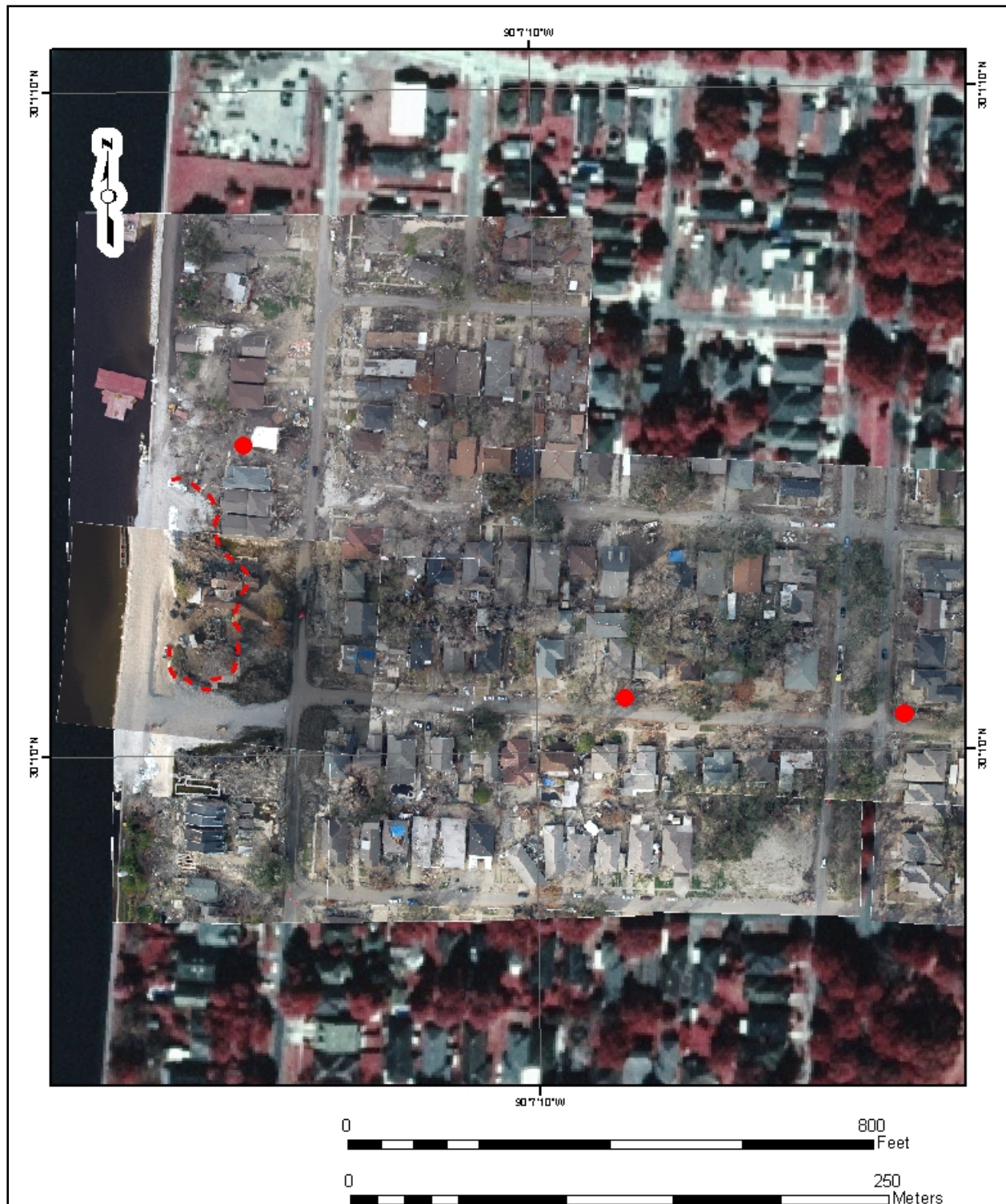
Figure 23a. November 2005 photograph showing locations where the grey lake clay and overlying marsh contact was observed. The accompanying photographs show close-up views of the swamp/marsh/lacustrine stratigraphy. The presentation of sites in the accompanying photographs is in a west to east direction in the above photograph. Sites are designated as west (Figures 23b and 23c), center (Figure 23d), and east (Figures 23e and 23f).
