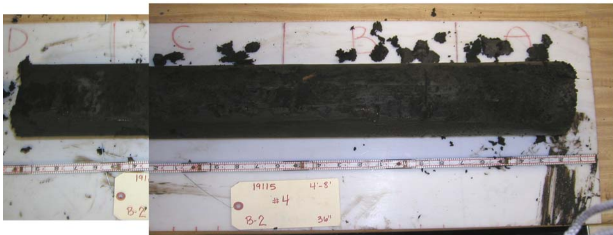
Figure 7c. Boring B-14, samples 2 (top), 3 (center), and 4 (bottom), 0.5 to 2 ft, 2 to 4 ft, and 4 to 8 ft, respectively. Top of samples are at right and bottom at left. Sample 2 from levee fill, and samples 3 and 4 are in the swamp/marsh environment--note the high water and the high organic content as indicated by the CHOA to CHOC designation (see Figures 1 and 7b). Presence of wood pieces and roots are common in samples. Samples from west edge of displaced levee section and are disturbed.
