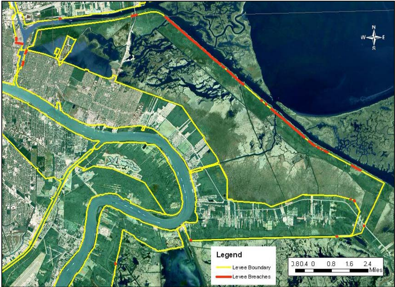
Figure 26. St. Bernard Parish breach locations.
