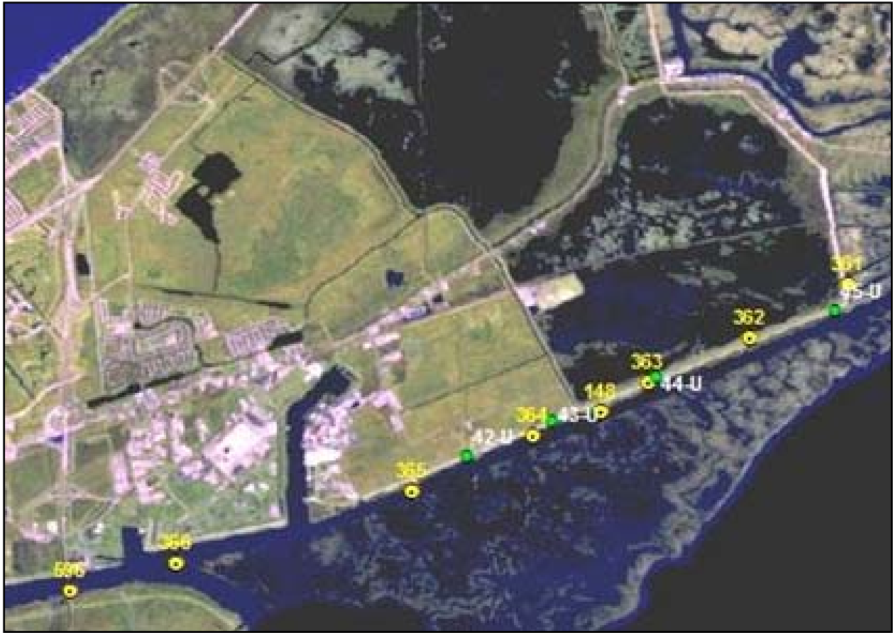
Figure 14. Location of undisturbed borings ( 42-U, 43-U, 44-U, 45-U) drilled in 2001 along the NOE Back Levee
