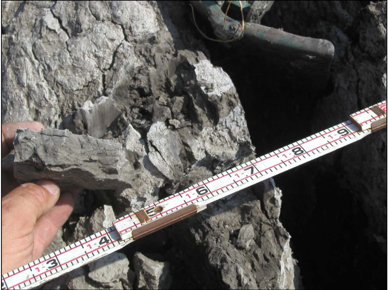
Figure 23f. Close-up view of the grey lake clay from the soil block at the intersection of Spencer Avenue and north bound lane of Fluer de Lis.
