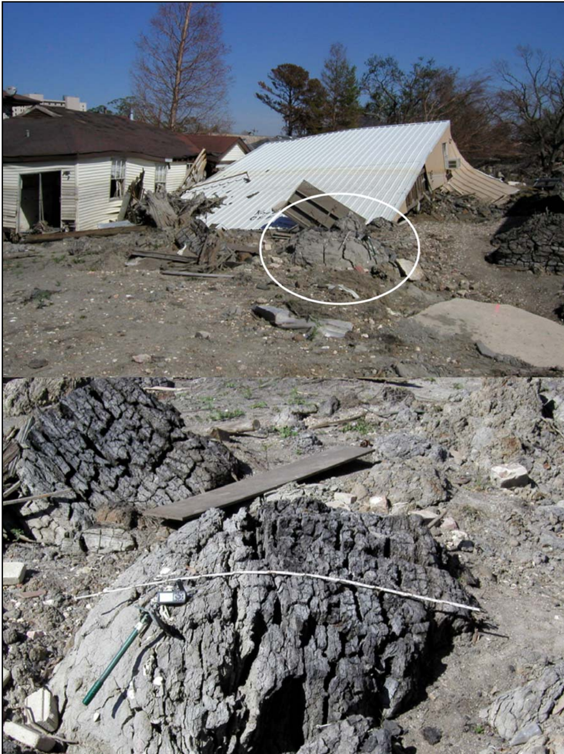
Figure 23b. Block of soil from levee foundation near boring 64, showing the intact marsh and lacustrine contact. A six foot folding rule is stretched across the soil mass. Upper photo shows the general setting (see Figures 22 and 23a for location). Lower photo shows block with about 3 ft of marsh and 3 ft of grey lacustrine clay. Whole shells are embedded within the grey lacustrine soils near the base of the soil block, where the shovel tip is located. Close-up view is shown in Figure 23c.
