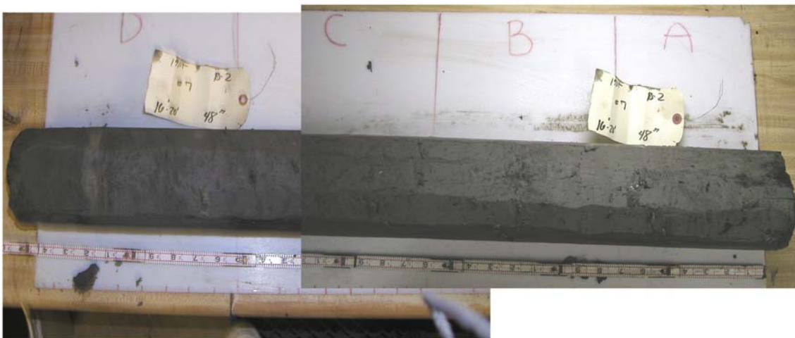
Figure 7d. Boring B-14, samples 5 (top), 6 (center), and 7 (bottom), 8-12 ft, 12-16 ft, and 16-20 ft; respectively; sample 5 is from swamp/marsh environment, and samples 6 and 7 are from the lacustrine environment. Note the darker color, higher water and organic contents for sample 5 (Figure 7b, CHOA to CHOC). Lighter grey color, lower water and organic contents, shell fragments (white specs), and laminations and lenses of silt and/or fine sand are diagnostic of lacustrine (lake) sediments
