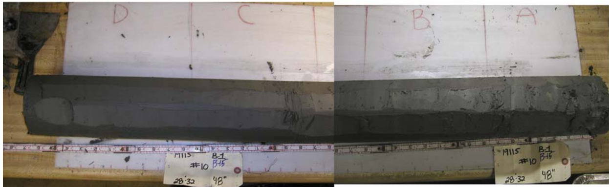
Figure 8e. Boring B-15, samples 8 (top), 9 (center), and 10 (lower); depths from 20 to 24 ft, 24 to 28 ft, 28 to 32 ft, respectively. See boring and lab logs in Figures 8a and 8b for descriptions. All three samples are from the lacustrine stratigraphic unit. This unit characterized by grey clay, note the presence of light colored silt and fine sand lenses, laminations, and thin beds. Also, note the water content in boring and lab logs ranges between 37 and 89 percent. Samples are merged in photographs above by bedding features between adjacent photos, and may not align with the sample board in background.
