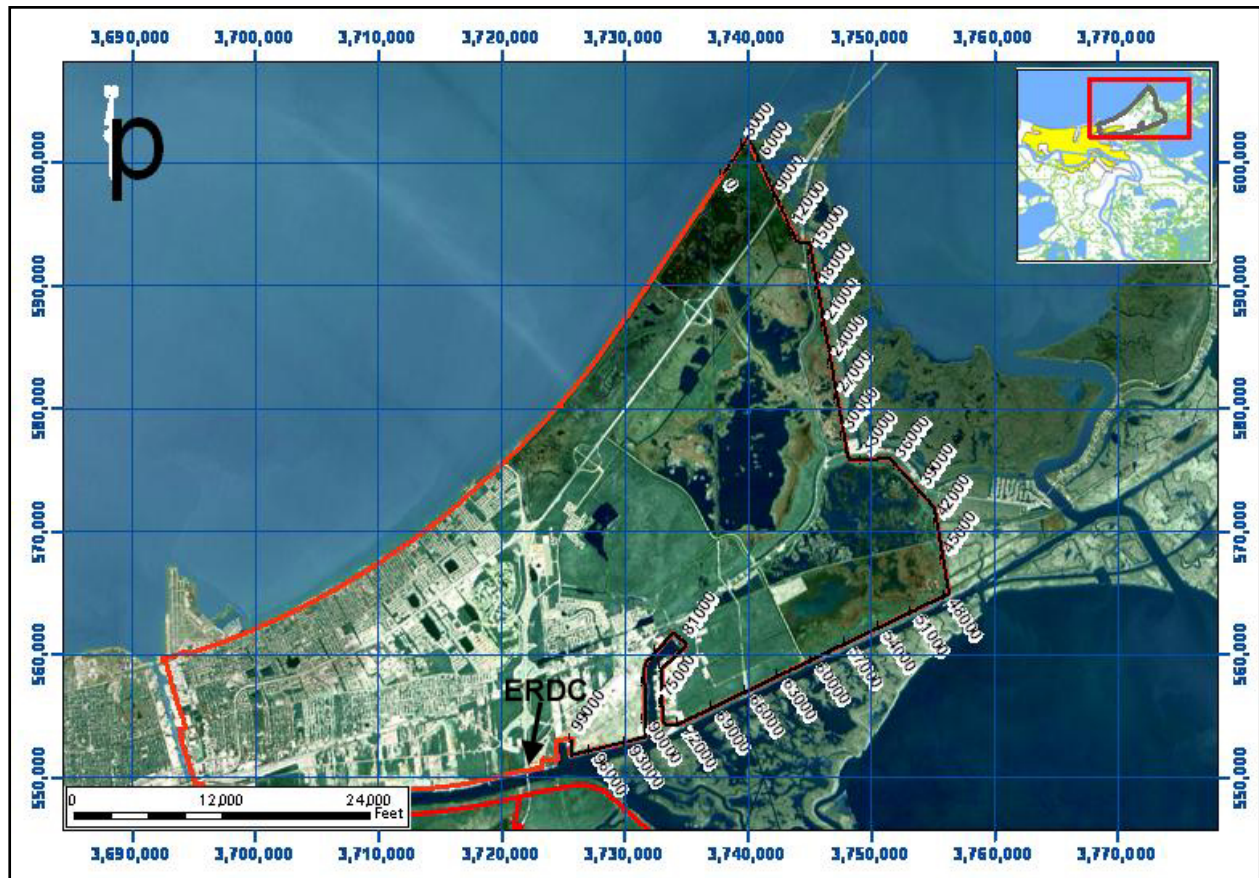
Figure 8. LIDAR stationing used in this report, starting at Lakefront levee and ending at the Michoud Slip along the GIWW. ERDC erosion test location under the I-510 Bridge is shown.
