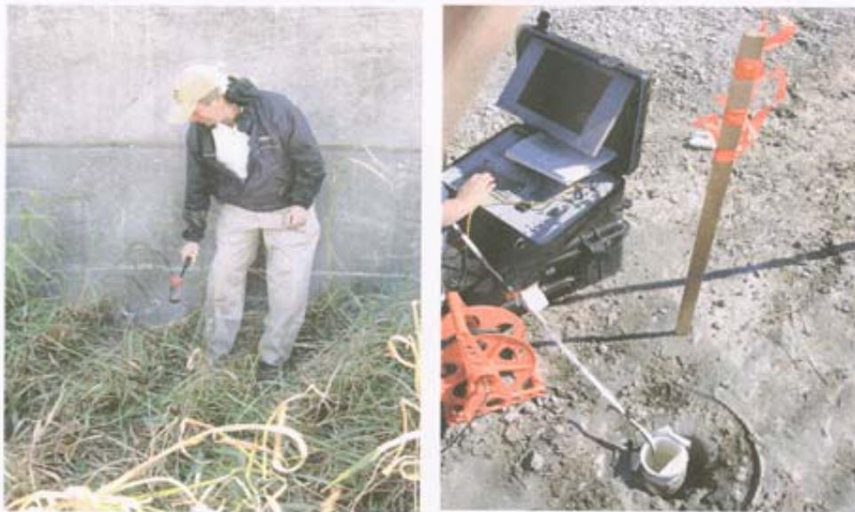
Figure 2 - Photographs of impacting Wall of IHNC Levee at South Borehole of South Breach and Freedom Data PC at Cased Borehole with Hydrophone Receiver Downhole
