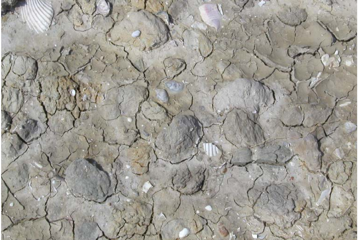
Figure 14-126. Exposed Soil Layer at Horizontal Scour Surface Appears to be In-Situ Fat Clay With Embedded Shell Hash, Possibly an Exposed Estuarine Deposit
