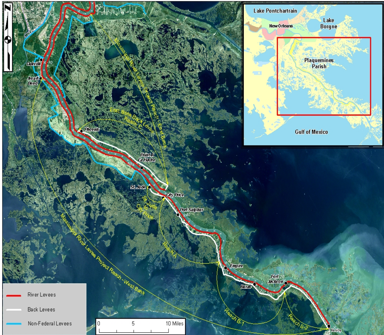
Figure 14-2. Extent of NOV Hurricane Protection in Plaquemines Parish. The NOV consists of five distinct reaches; Reach C, Reach St. Jude to City Price, Reach A, Reach B-1 and Reach B-2
