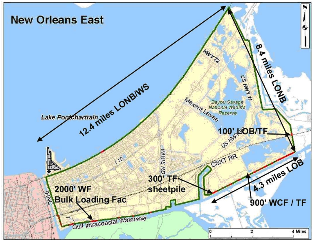
Figure 14-7. New Orleans East IPET Characterization of Damages
