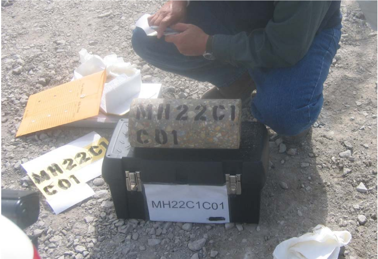
Figure 15-10. Cylindrical Core from Wall Panel H22
