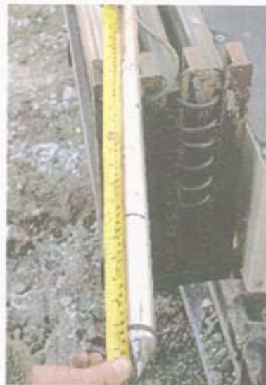
Photo 2 - Seismic Cone Penetrometer Tool with Bearing pressure at tip followed by pore pressure ring followed by skin friction sleeve followed by bi-axial horizontal geophones
