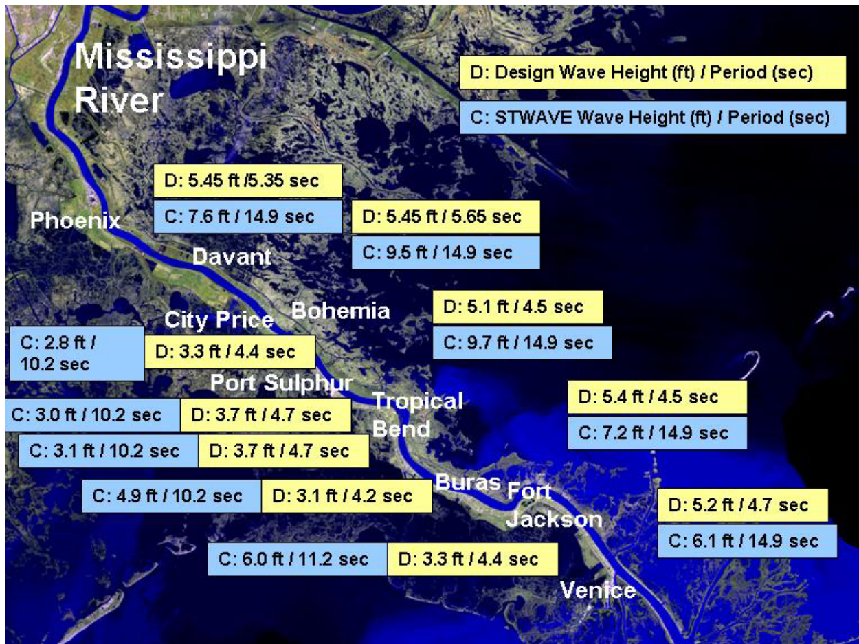
Figure 87. Wave maxima along hurricane protection levees in Plaquemines Parish
