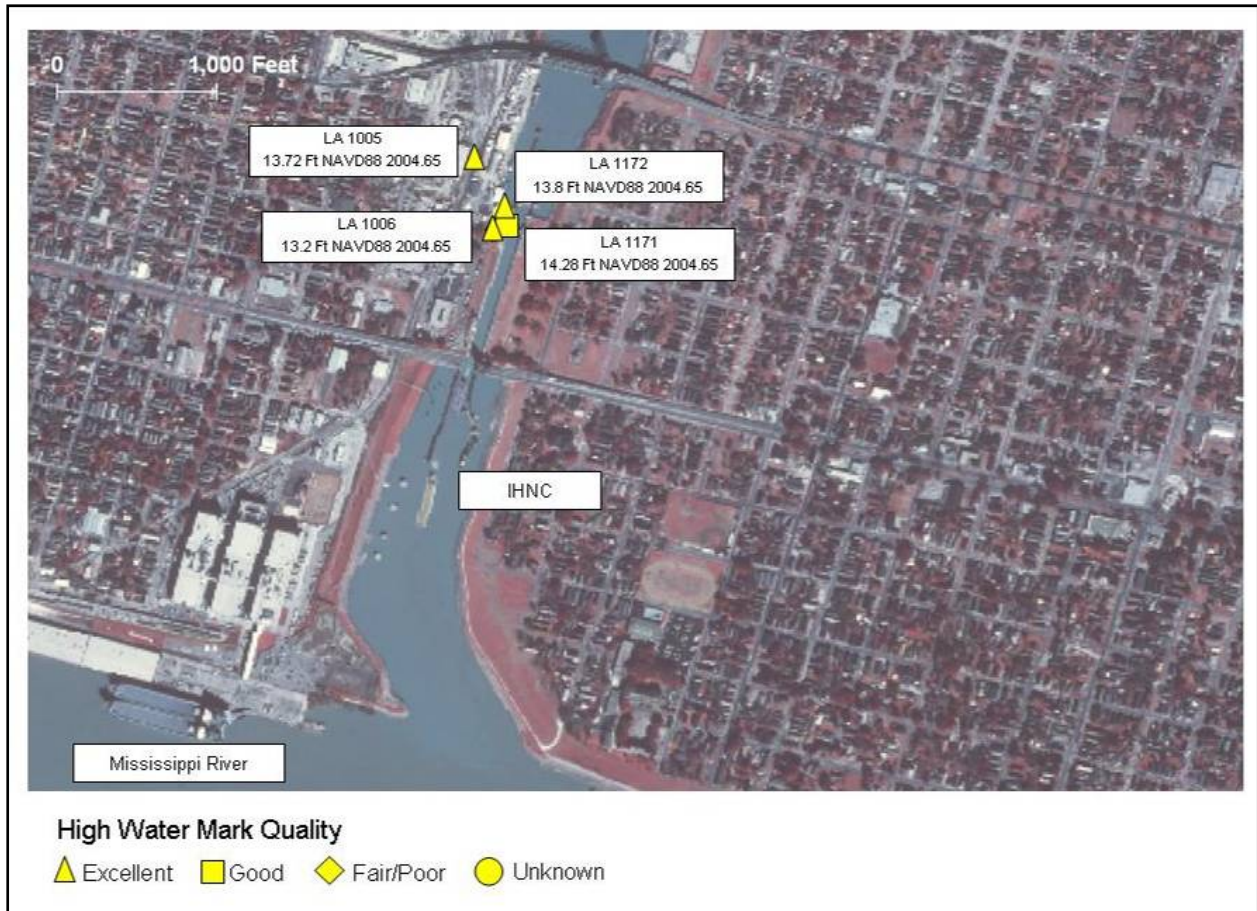
Figure 2. Sample image of the Inner Harbor Navigation Canal and Lock vicinity showing locations of HWMs and water elevation for each mark.
