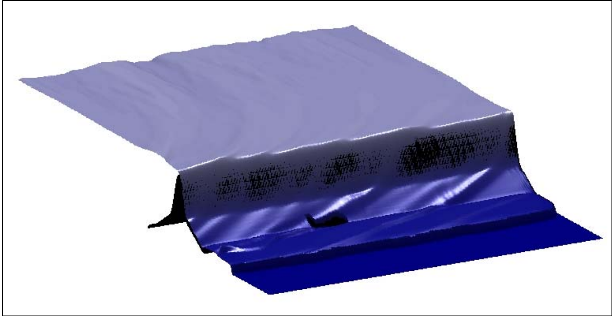
Figure 185. Side angle view of numerical waves overtopping the levee near the Paris Road Bridge. The levee is shown as the submerged black shape. View is looking towards the southwest; waves are from the east (left side of image).
