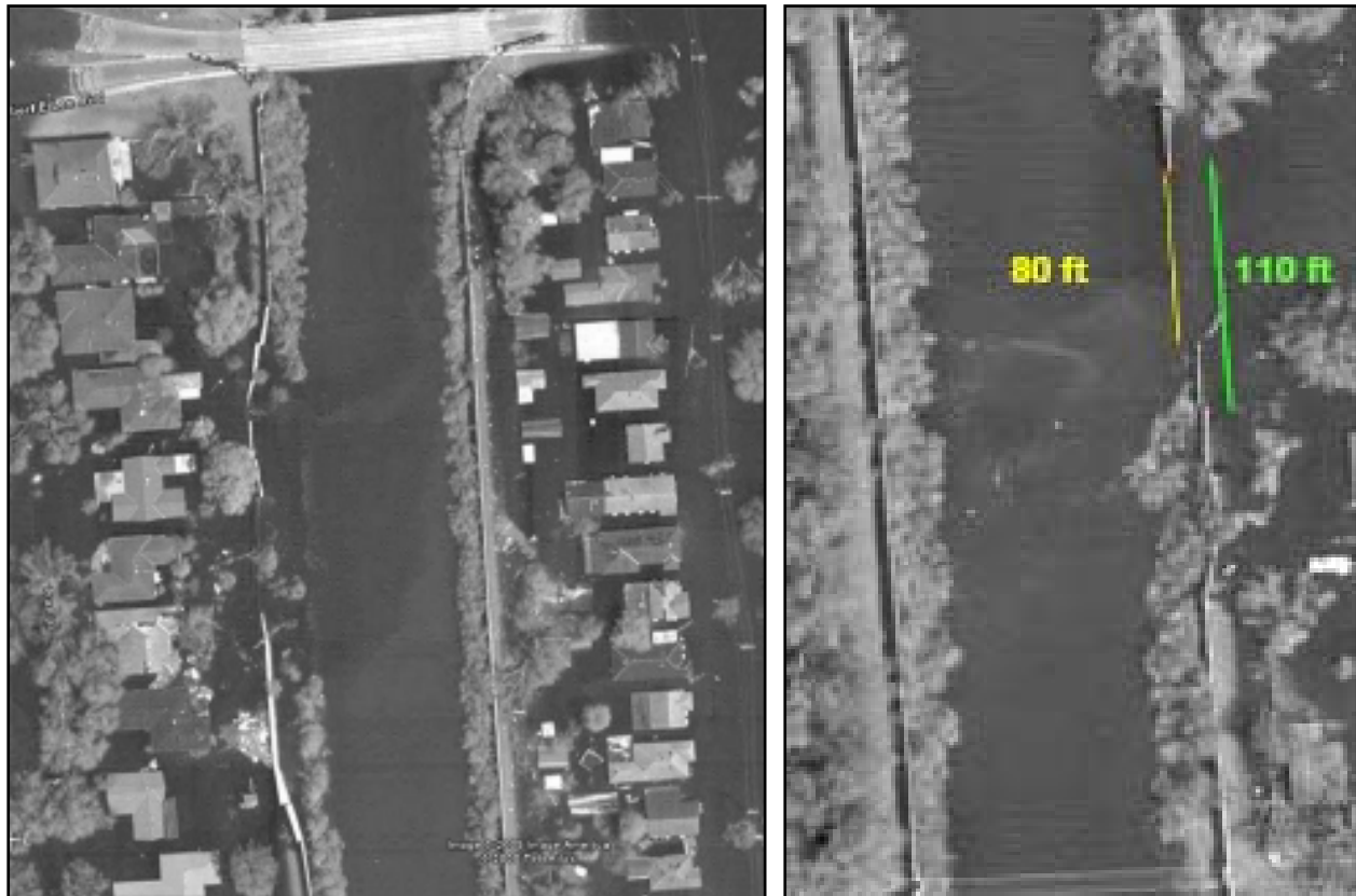
(a) North breach near Robert E. Lee bridge
