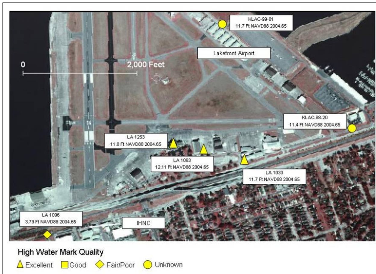
Figure 9. Lake Pontchartrain entrance to IHNC, Lakefront Airport, showing locations of HWMs and water elevation for each mark.
