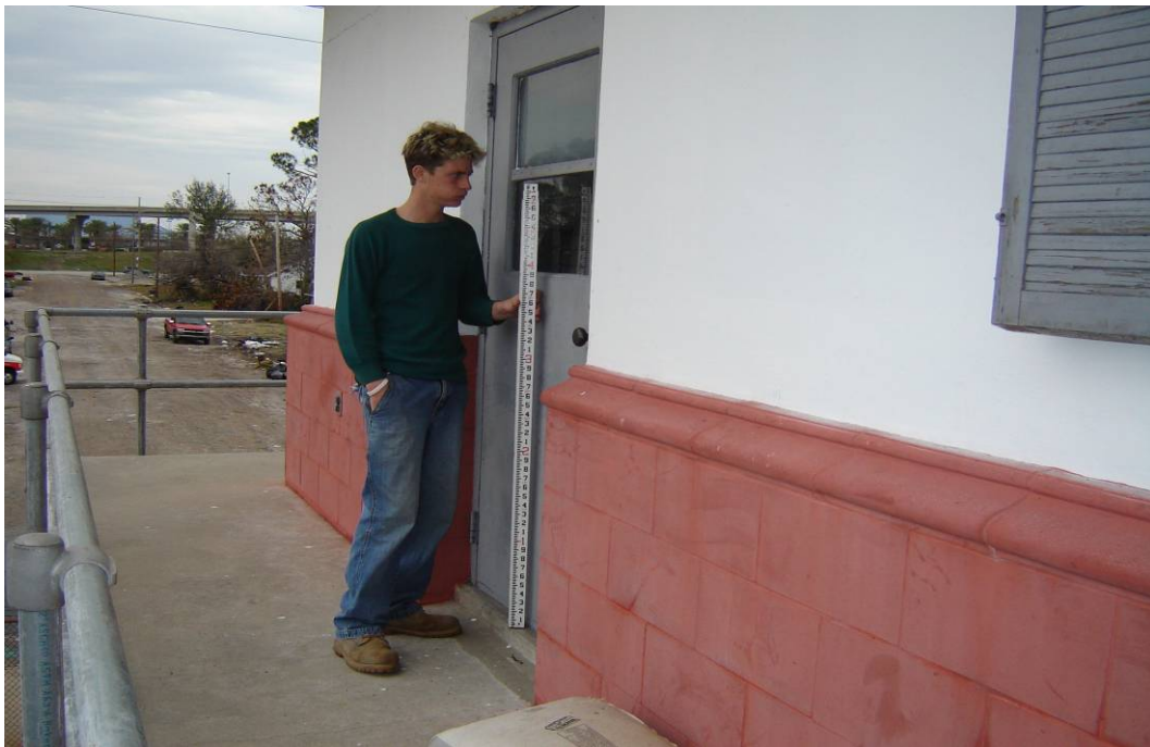
Finished Floor = 14.85 feet NAVD88(2004.65) Field Book 060851
