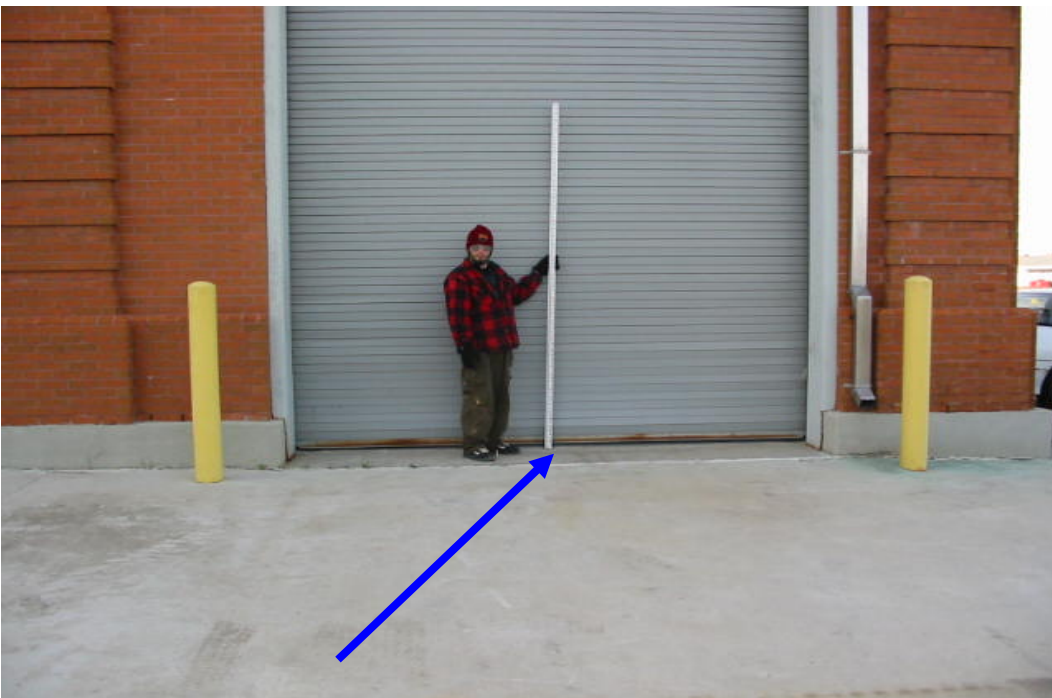
OP 19 Finished Floor #2 = -4.33 feet NAVD88(2004.65) Field Book 060851
