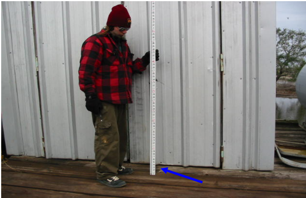
Finished Floor #1 = 7.81 feet NAVD88(2004.65) Field Book 060852
