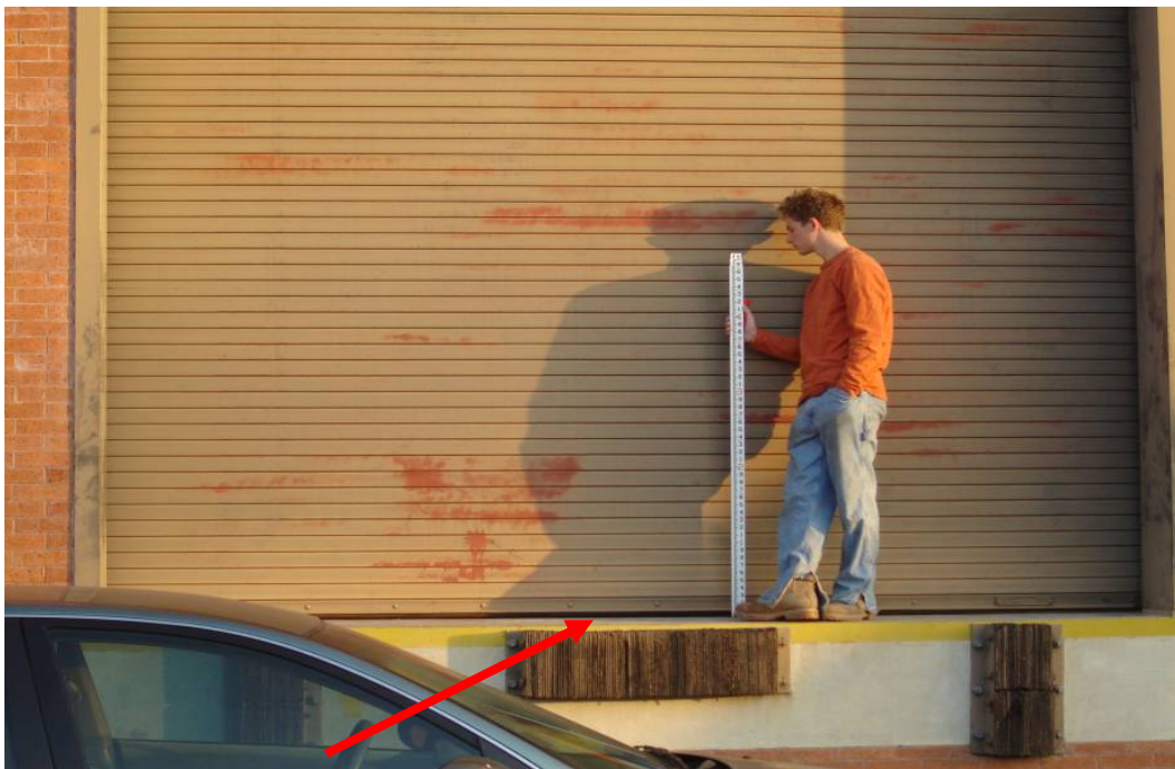
Finished Floor #3 = 4.75 ft, NAVD88(2004.65) Bk.060852, Pg. 40
