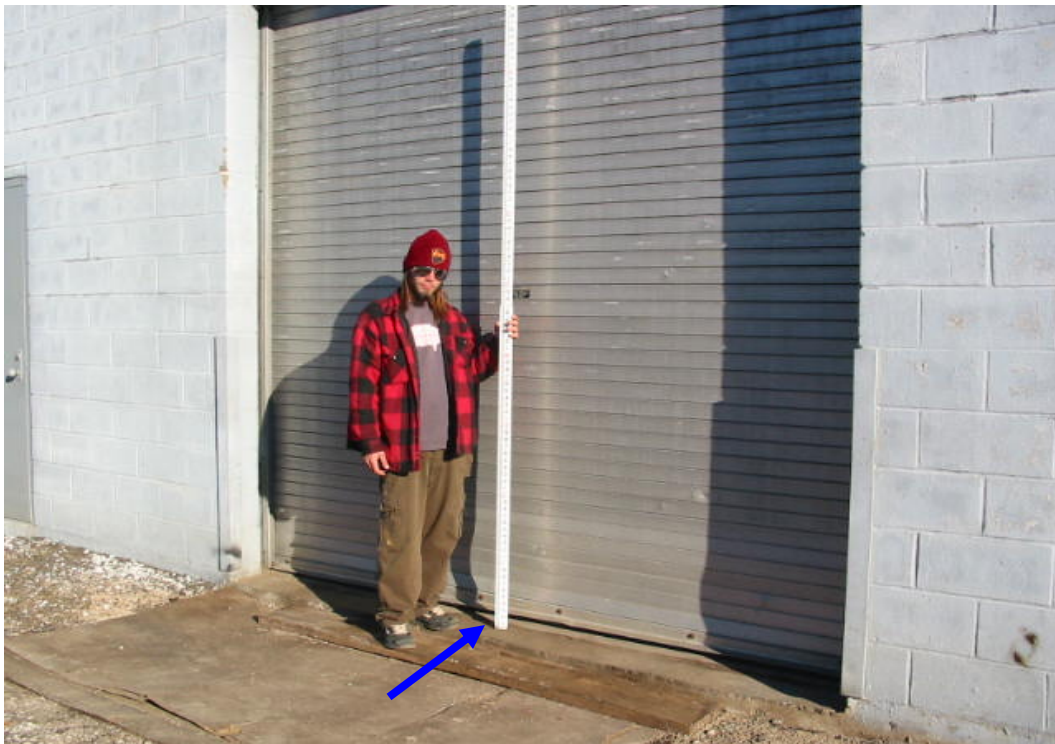
Finished Floor = 4.75 feet NAVD88(2004.65) Field Book 060851
