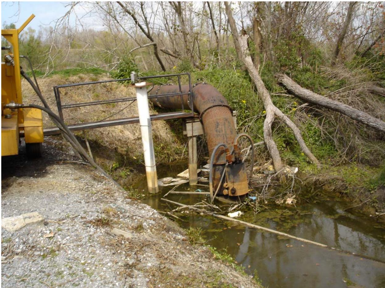
Figure 23. Hydraulically Driven Submersible Pump
