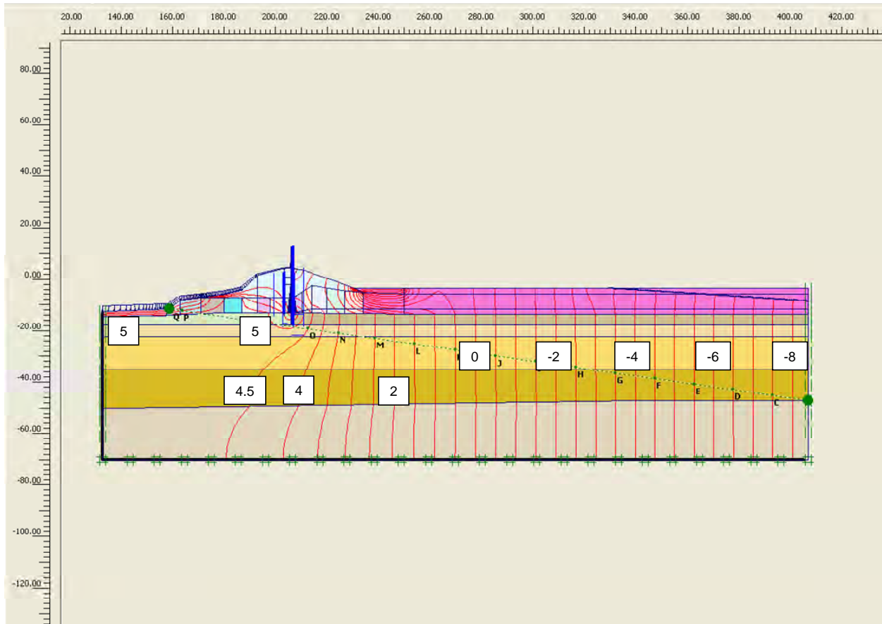
Figure 9-5. Equipotential Lines from a Steady State Seepage Analysis for Canal Water El 6 and a Crack to the Top of Beach Sand (El -12.9) on the Canal Side of the New Sheet Pile Wall
