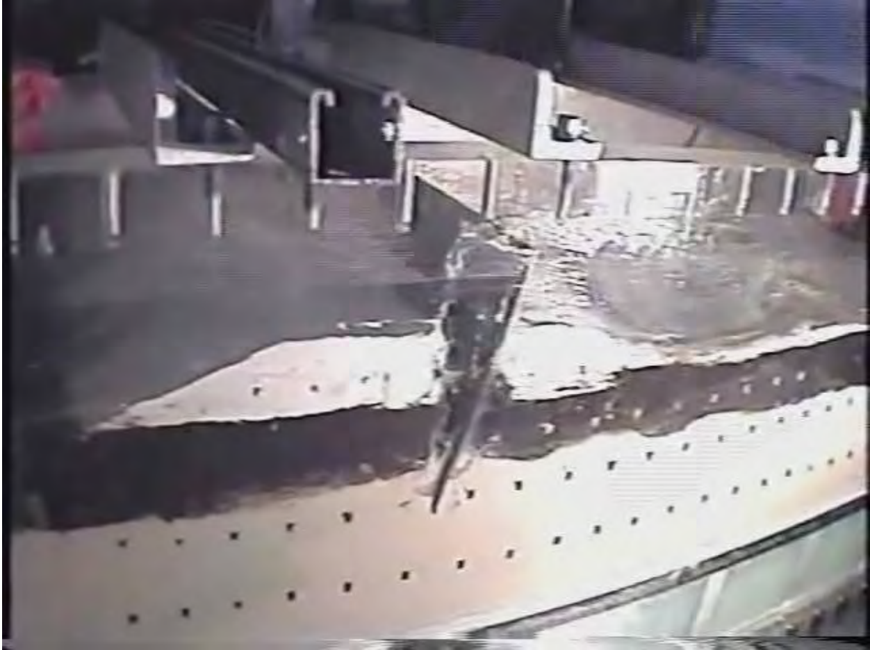
Figure 5.85d. View of ERDC London north model at flood level well into failure
