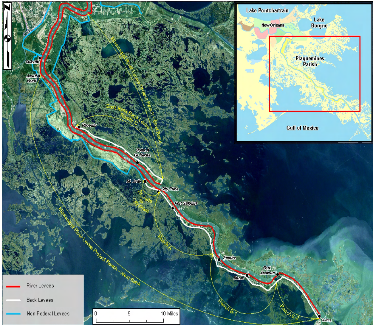
Figure 14-162. Plaquemine Parish Mississippi River Levees (MRL East Bank, MRL West Bank) and New Orleans to Venice Hurricane Protection Levees (St. Jude to City Price, Reach A, Reach B-1, Reach B-2, and Reach C) Project Reaches
