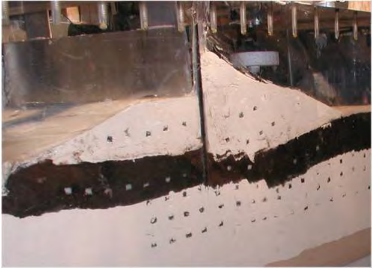
Figure 5.33. Bearing failure and multiple slip planes in the clay foundation caused by rapid construction on landward side, 17th Street Model 2
