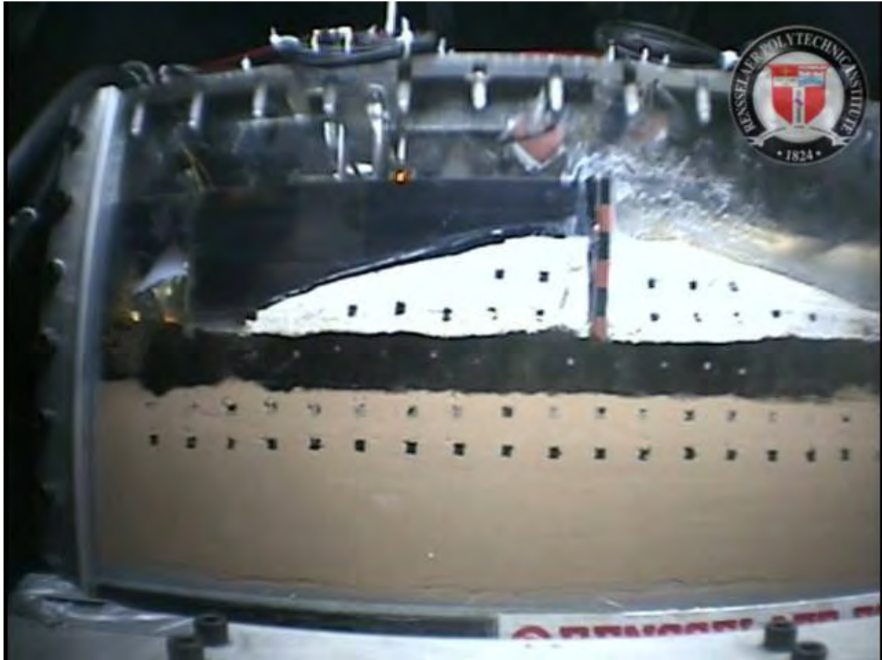
Figure 5.102e. View of RPI Orleans south model with water elevation raised above hurricane Katrina level showing movement of wall
