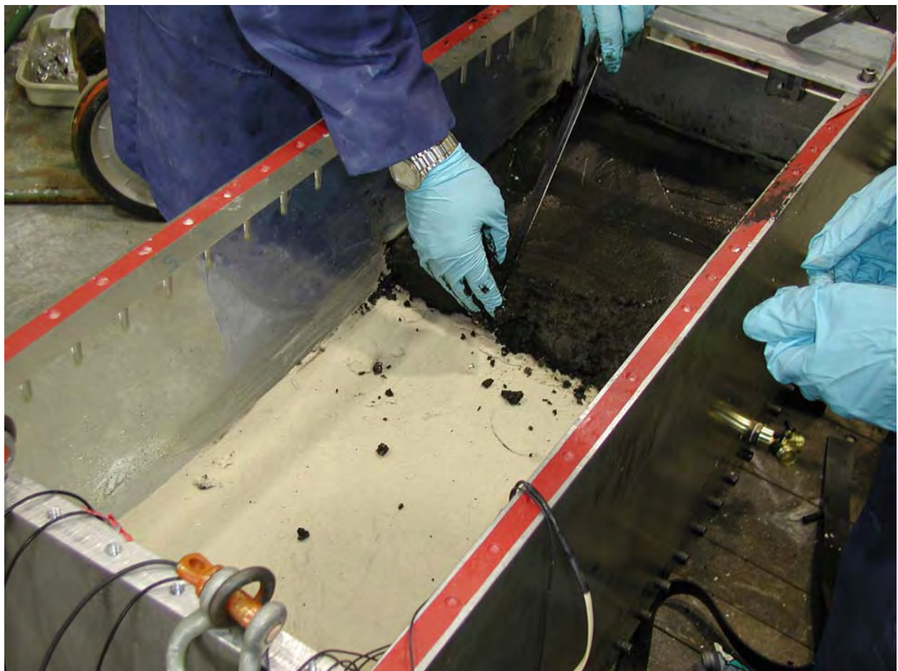
Figure 5.80. View of placement of swampy/marsh layer
