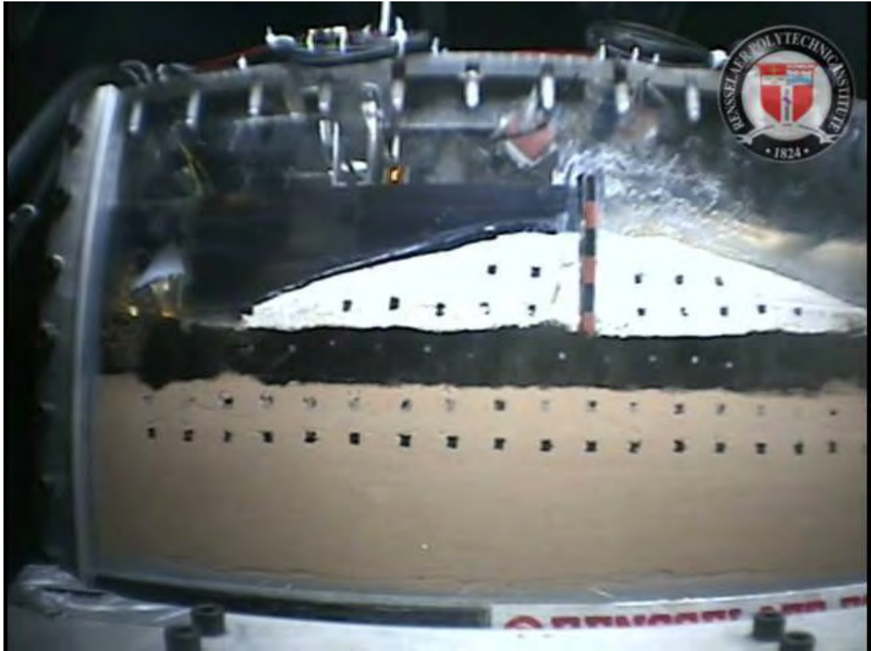
Figure 5.102d. View of RPI Orleans south model with water elevation raised above hurricane Katrina level to near top of wall
