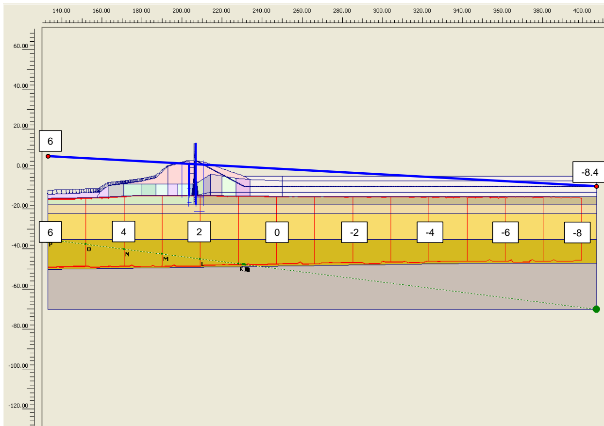
Figure 9-6. Equipotential Lines Based on a Linear Phreatic Surface for Canal Water El 6 and a Crack to the Top of Beach Sand (El -12.9) on the Canal Side of the New Sheet Pile Wall
