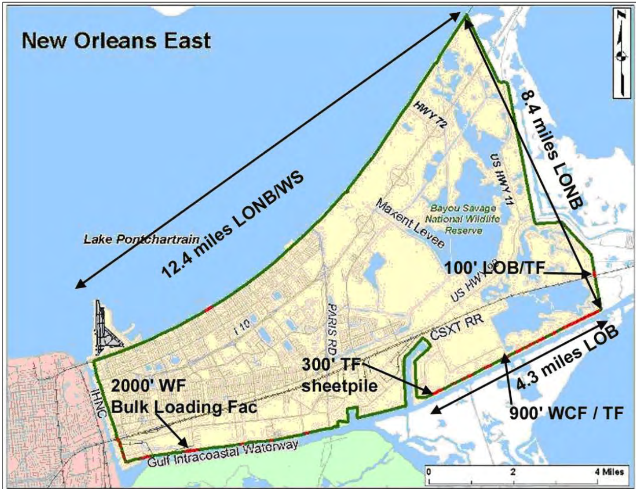
Figure 14-7. New Orleans East IPET Characterization of Damages
