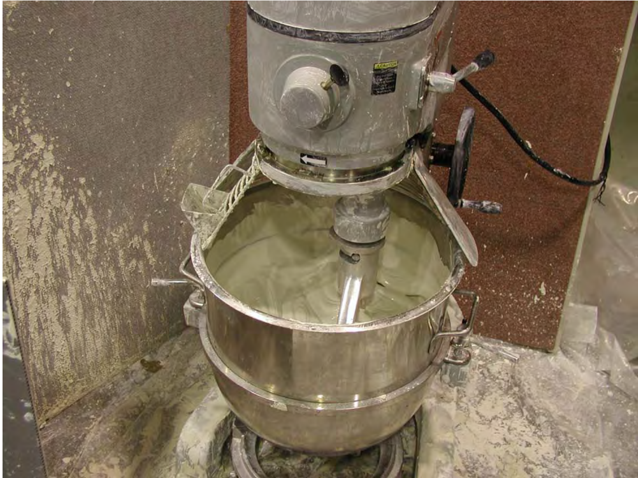
Figure 5.42. View of the clay mixing process
