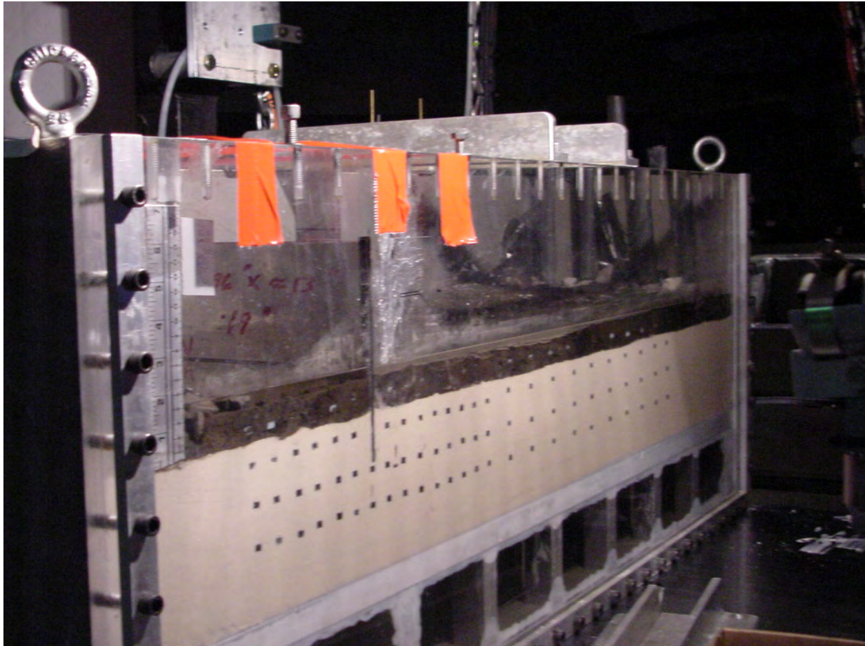
Figure 5.64. View of the ERDC model with sand and swampy/marsh layer
