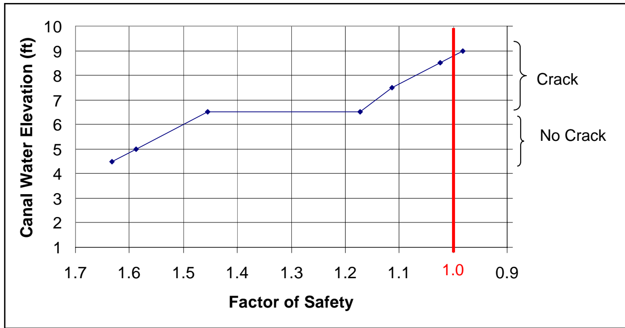
Figure 6-41. Factor of Safety Versus Canal Water El (Complete SSI results)
