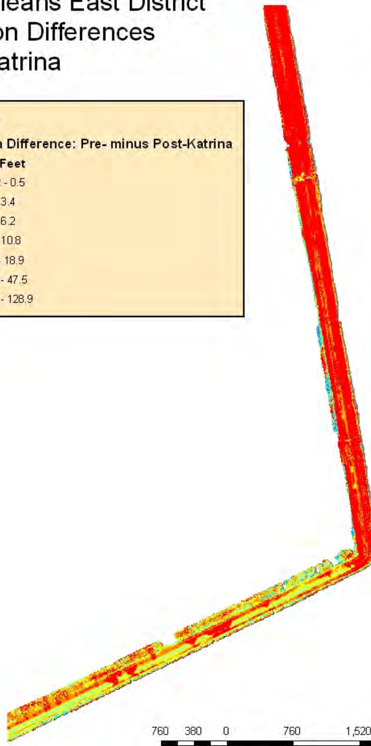
Figure 18-5. Hillshading from pre-Katrina LIDAR minus post-Katrina LIDAR, southeast corner of New Orleans East Basin. Figure created from raw LIDAR data, thus noise and outliers not removed from dataset. Red areas indicate less than 0.5 ft of scour
