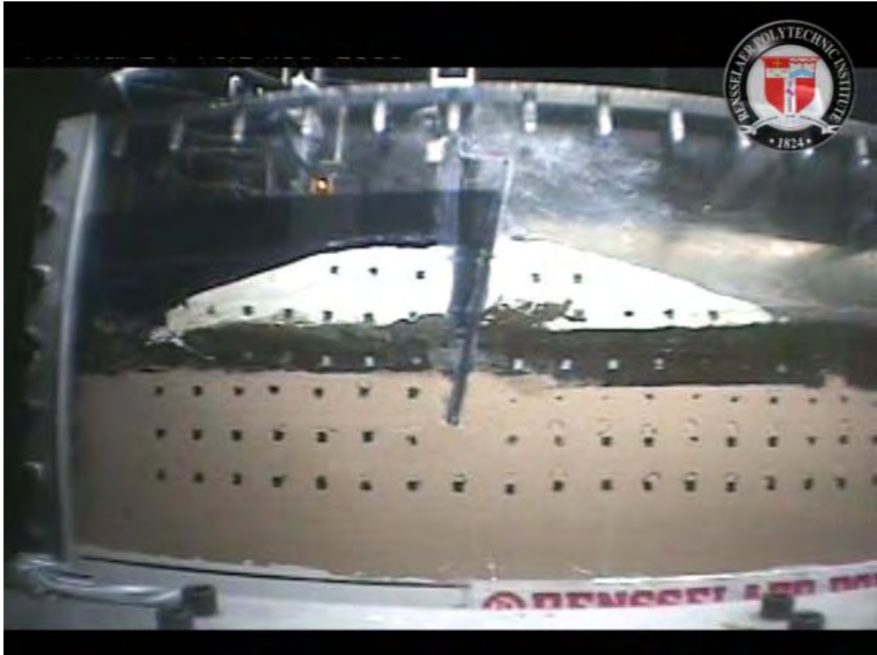
Figure 5.77e. RPI London south model in failure showing rotation of wall
