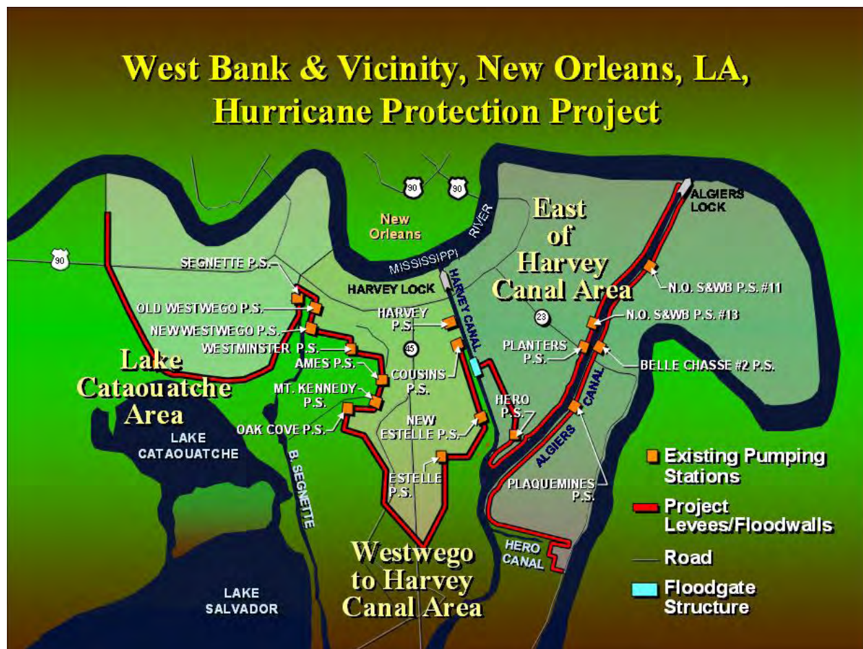
Figure 30. Hurricane protection project, West Bank and Vicinity, New Orleans, LA
