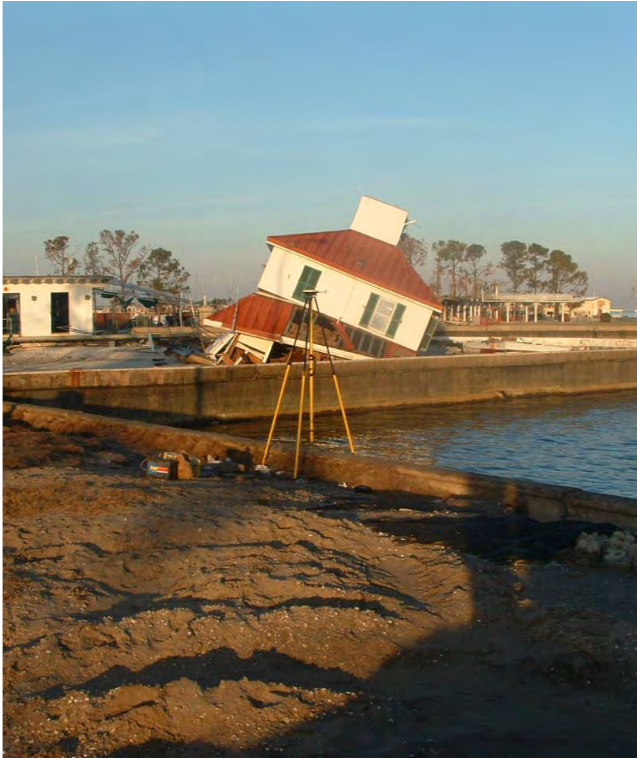
Figure 34. IPET GPS surveys in December 2005 at Benchmark ALCO on seawall bulkhead at US Coast Guard station vicinity NOAA New Canal gage (3001, Inc)
