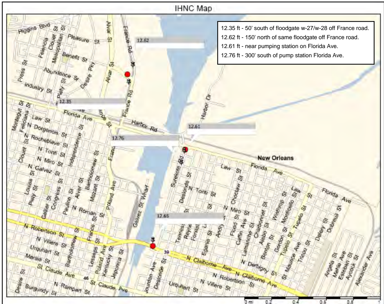
Figure 51. Selected Post-Katrina Elevations on IHNC Floodwalls
