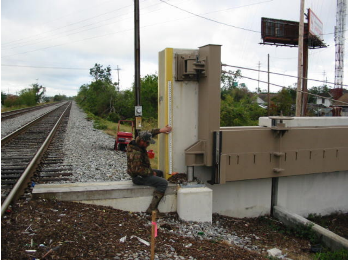
HWM OP-03 & London RR Gate – Survey arrow = 10.041' ft NAVD88 (2004.65) Bk. 060851, Pg. 19
